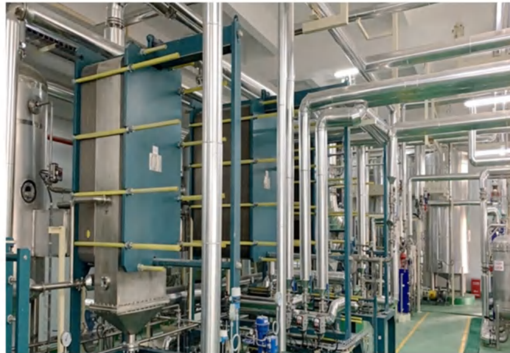
Evaporation capacity: 5t/h Evaporation process: MVR+TVR Multi-effect Fluid: Mannitol Final concentration: 45% Main material: SS316L
