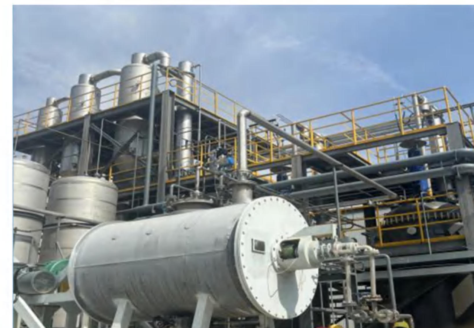
Evaporation: 2.5t/h Process: Double-effect tube force circulation+single still Material: CaCl 2 , MgCl 2 , KCl, NaCl Final concentration: Crystallization Main material: TA2
