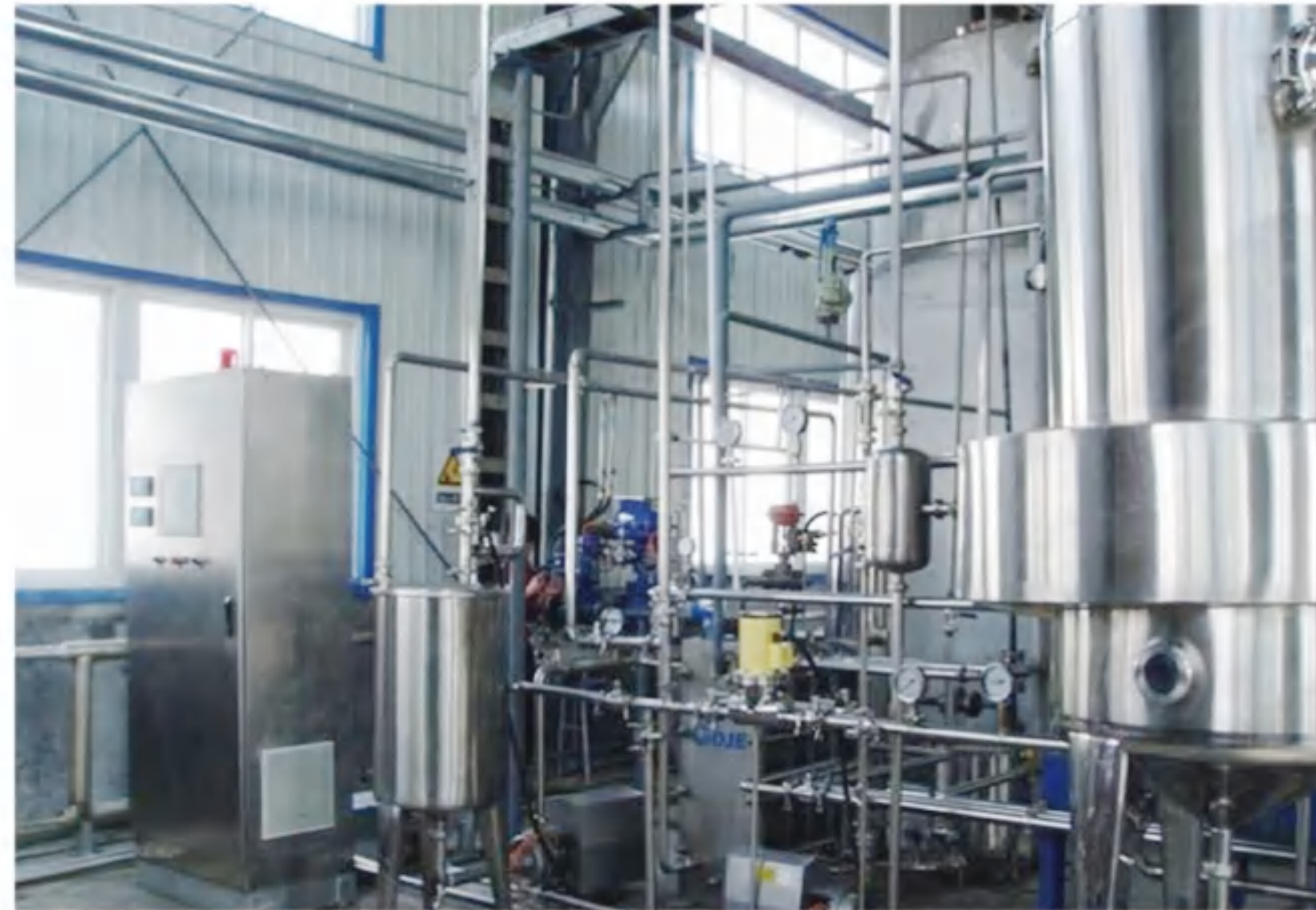
Evaporation capacity: 3t/h Evaporation process: Three effect Fluid: Sorbitol Final concentration: 70% Main material: SS304
