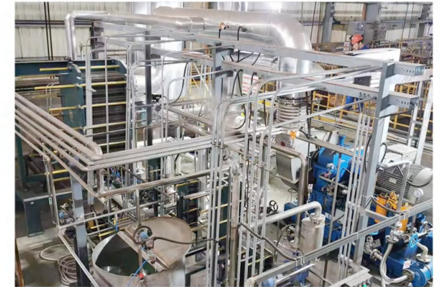
Evaporation capacity: 2.6t/h Evaporation process: MVR evaporation concentration Material: Pickling wastewater Main material: 254SMO
