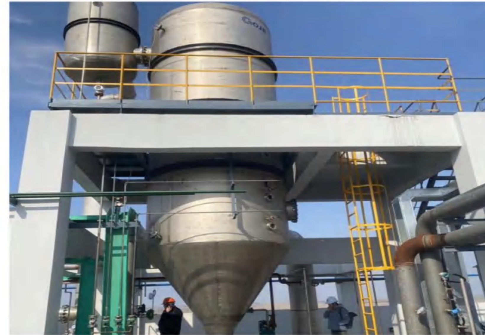
Evaporation: 5.4t/h Process: MVR tube forced circulation evaporation system Material: NaCl Final concentration: Crystallization Main material: TA2
