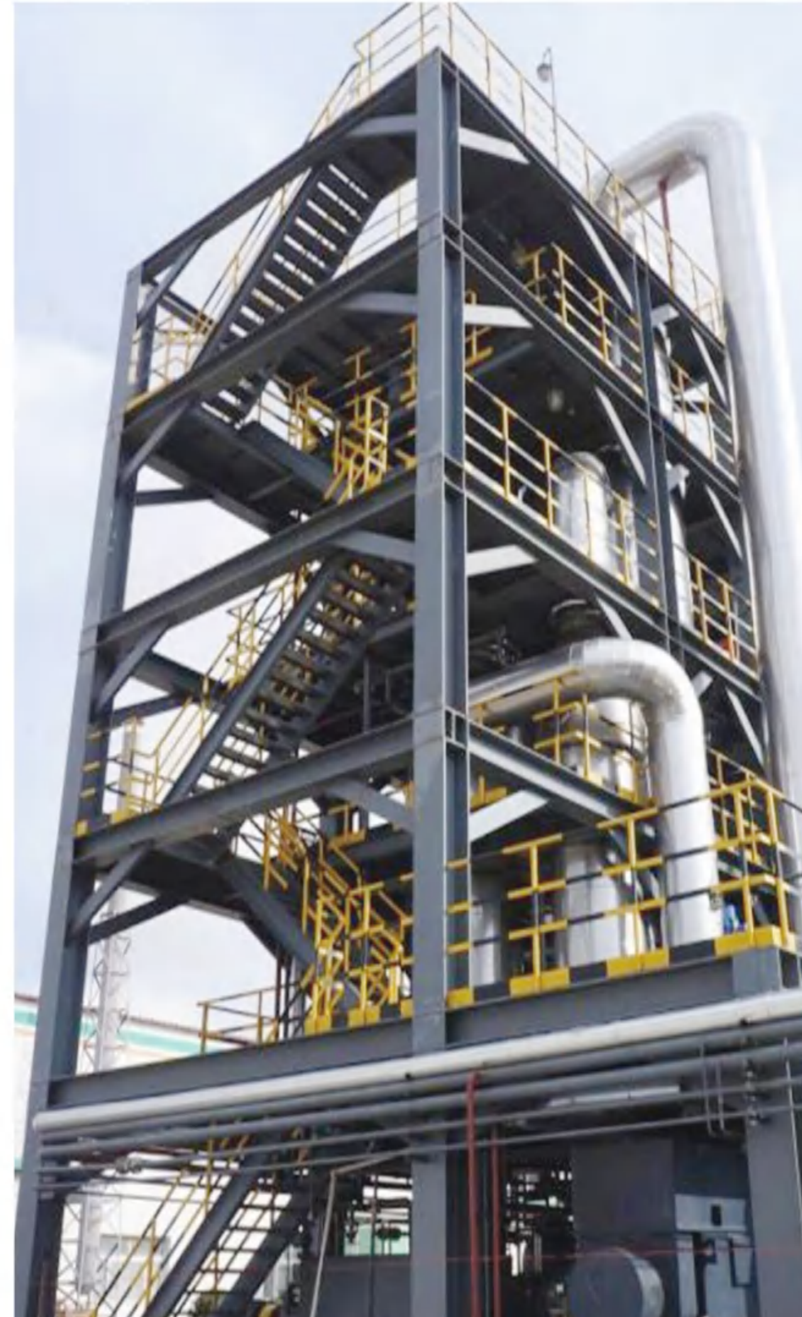
Evaporation capacity: 20t/h Evaporation process: MVR falling film+forced circulation Fluid: Ammonium sulfate solution Final concentration: Crystallization discharge Main material: SS316L
