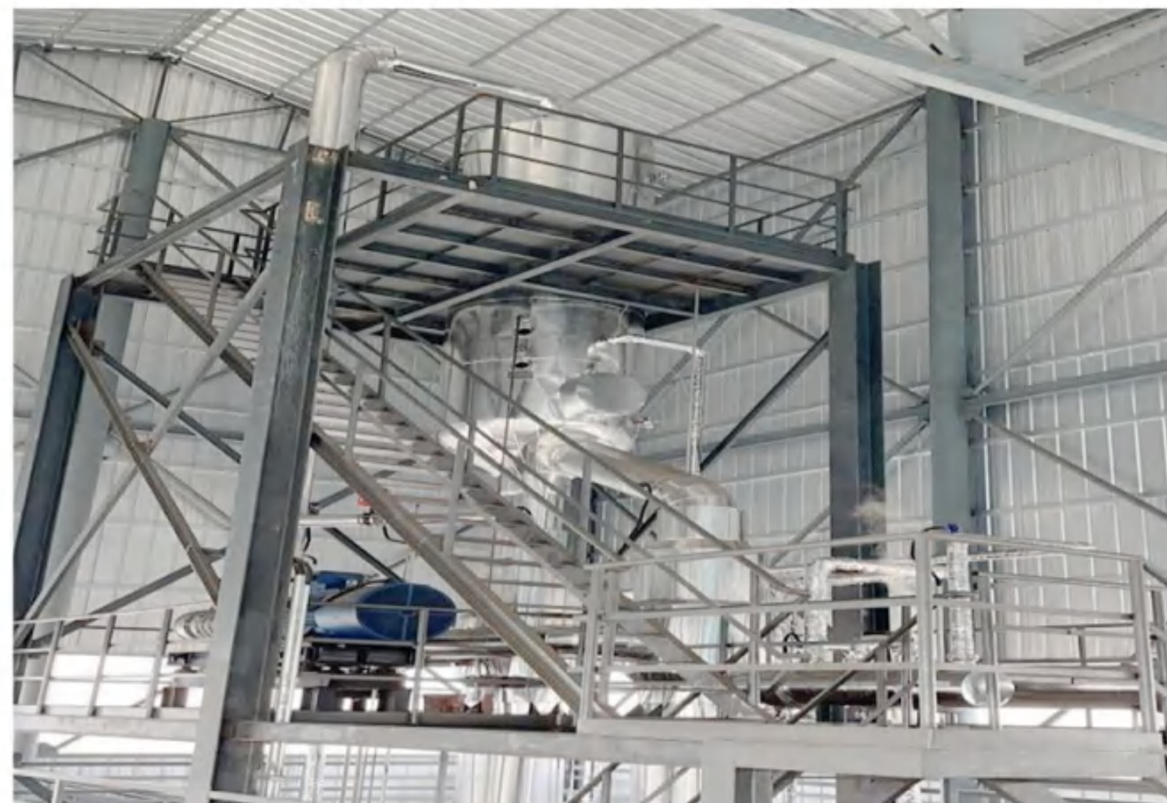
Evaporation capacity: 1.5t/h Evaporation process: MVR evaporation Fluid: Potassium fulvic acid Main material: SS304
