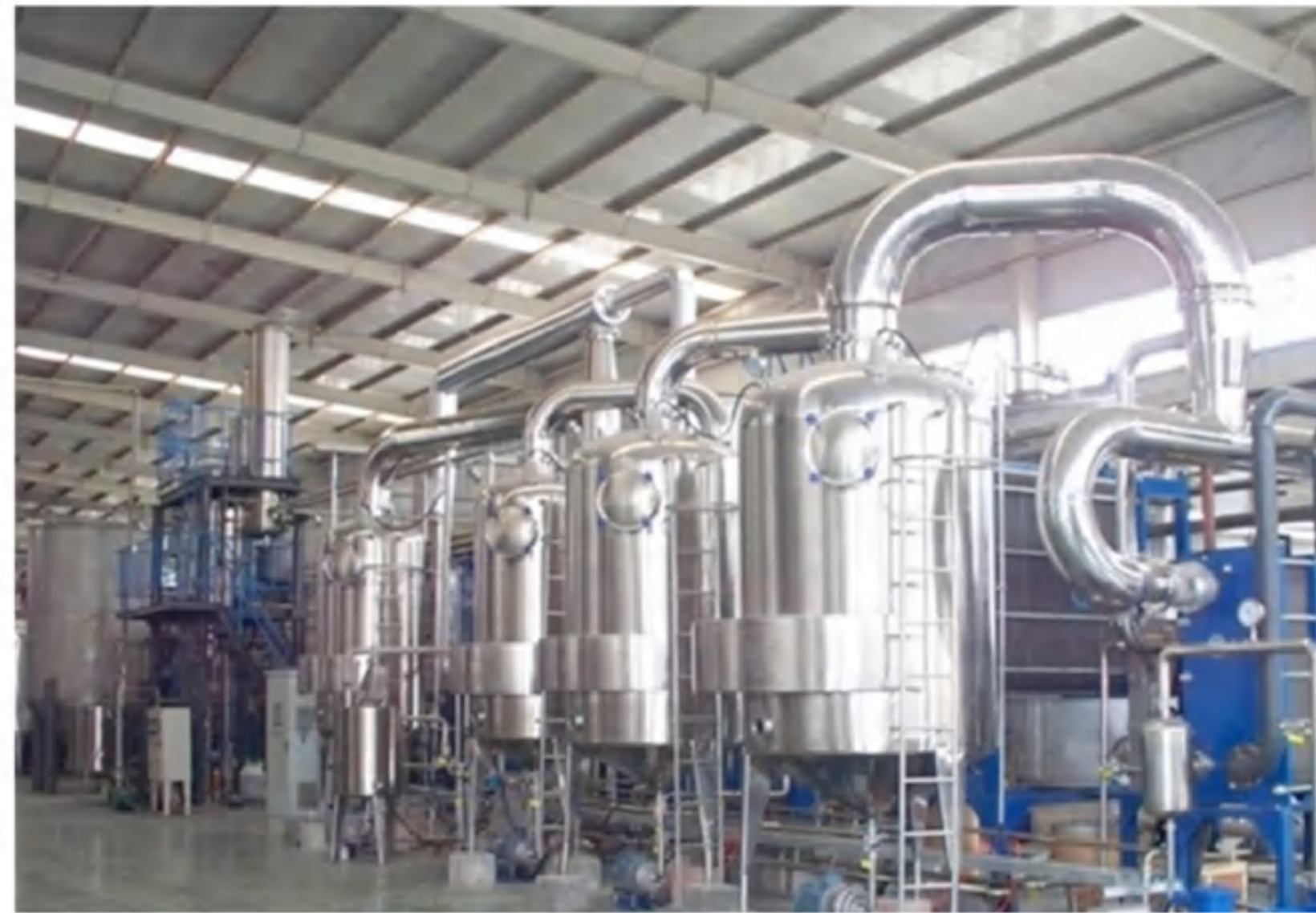
Evaporation capacity: 30t/h Evaporation process: Four effect Fluid: Maltose syrup Final concentration: 80% Main material: SS316L
