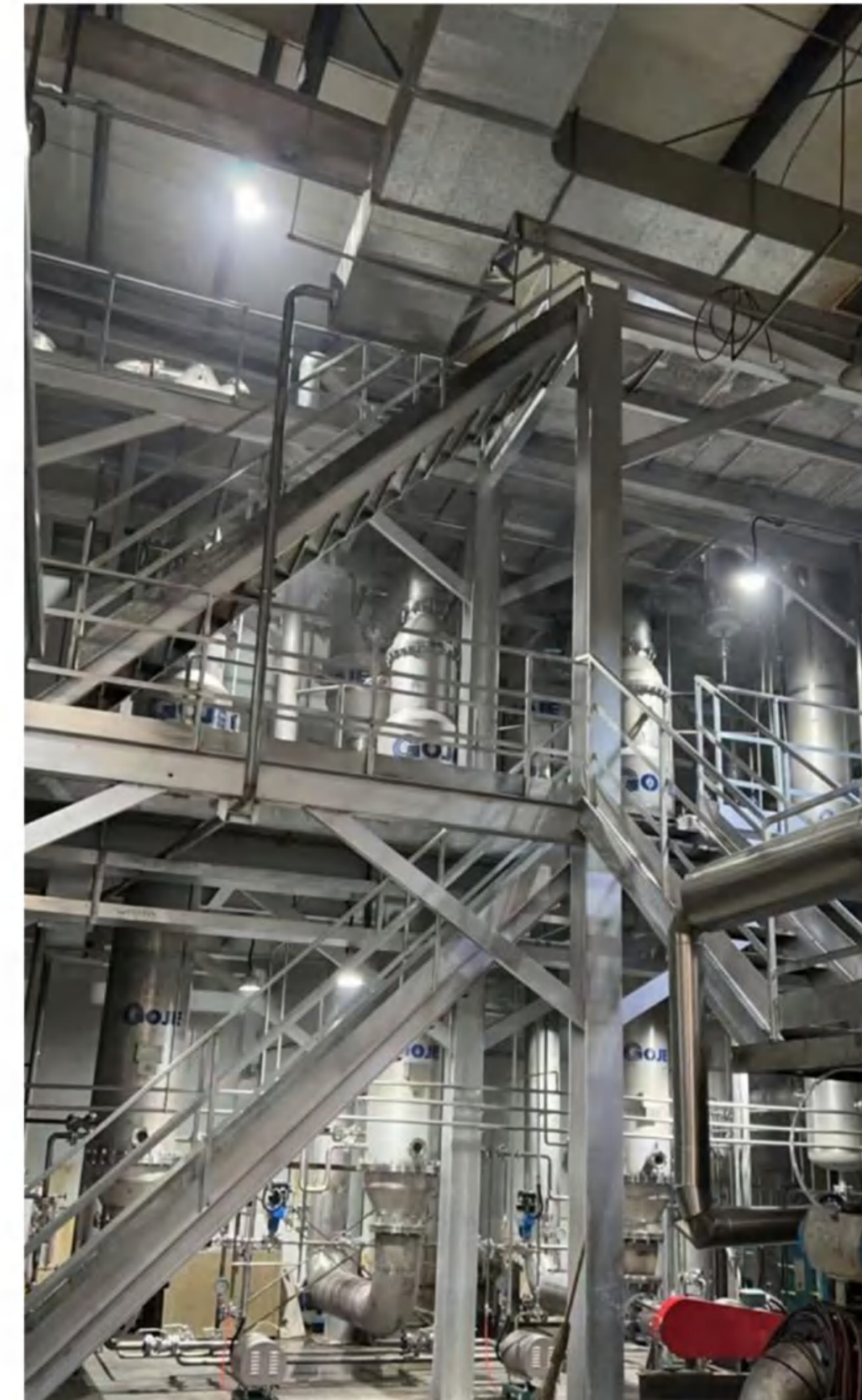
Evaporation: 2.5t/h Evaporation process: TVR four-effect tube Ingredients: bone broth solution Discharge concentration: 37.5% Main material: 30408
