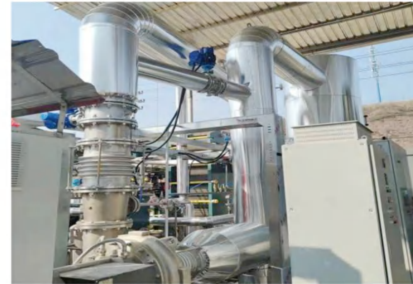
Evaporation capacity: 5t/h Evaporation process: MVR evaporation system Material: Sodium hydroxide Discharge concentration: 16.8% Main material: SS316L
