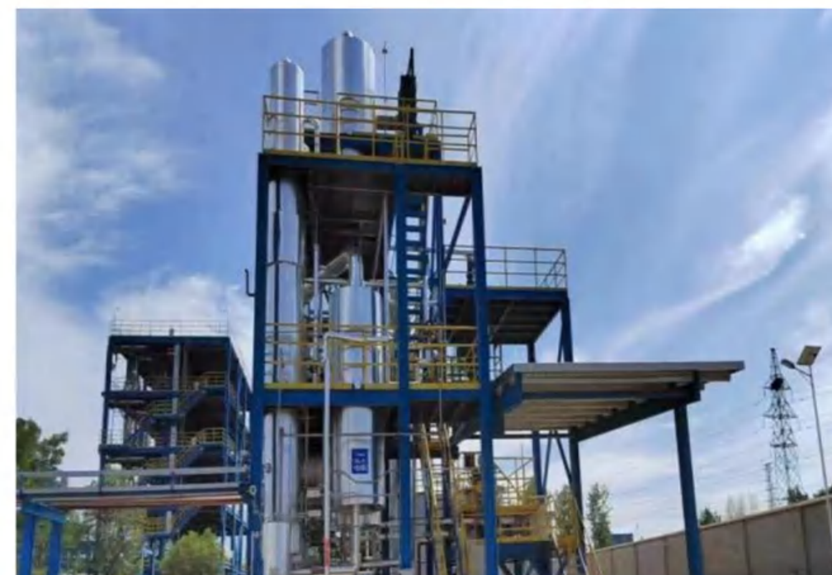
Evaporation capacity: 5t/h Evaporation process: Three effects Material: Sodium sulfate Main material: SS316L
