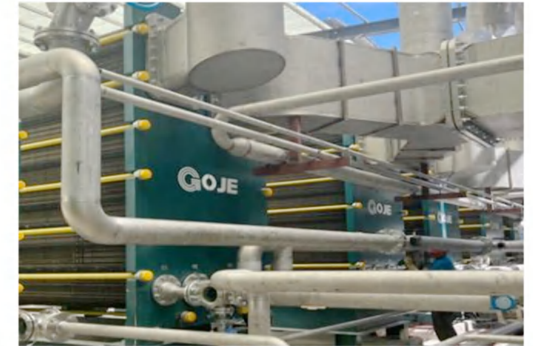
Evaporation capacity: 55+5t/h Evaporation process: MVR two-stage plate evaporation system Fluid: lactic acid Main material: TA1
