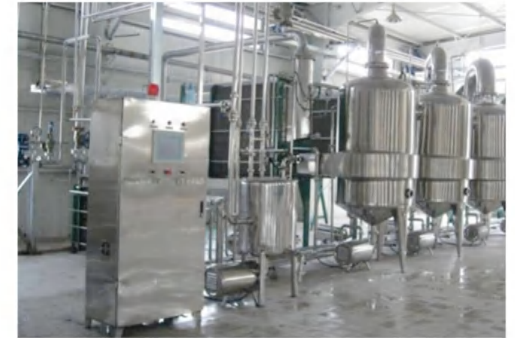
Evaporation capacity: 10t/h Evaporation process: Four effects Fluid: Mulberry juice Final concentration: 65% Main material: SS316L
