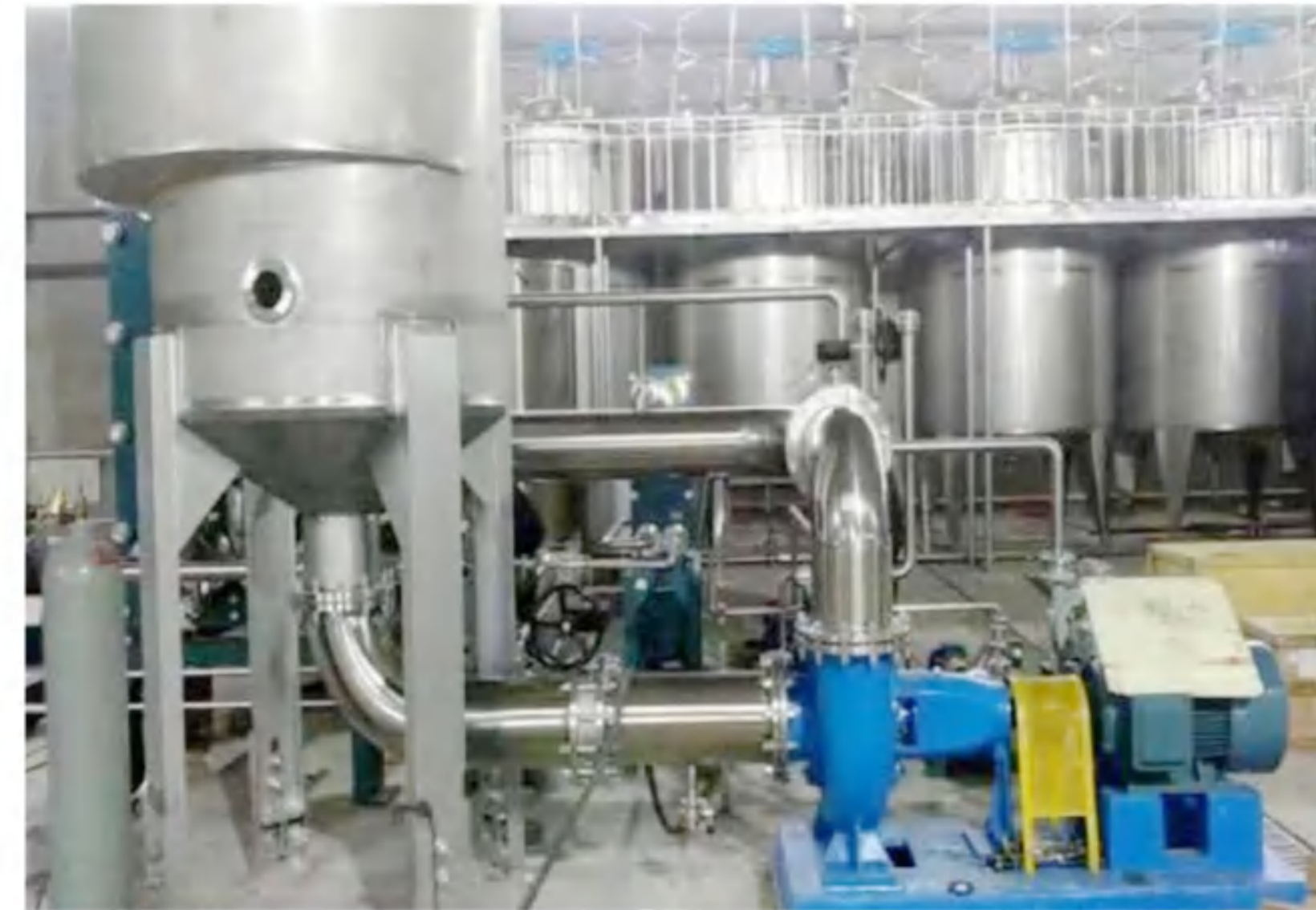
Evaporation capacity: 3t/h Evaporation process: MVR single effect Material: Blood peptide solution Final concentration: 41% Main material: SS316L
