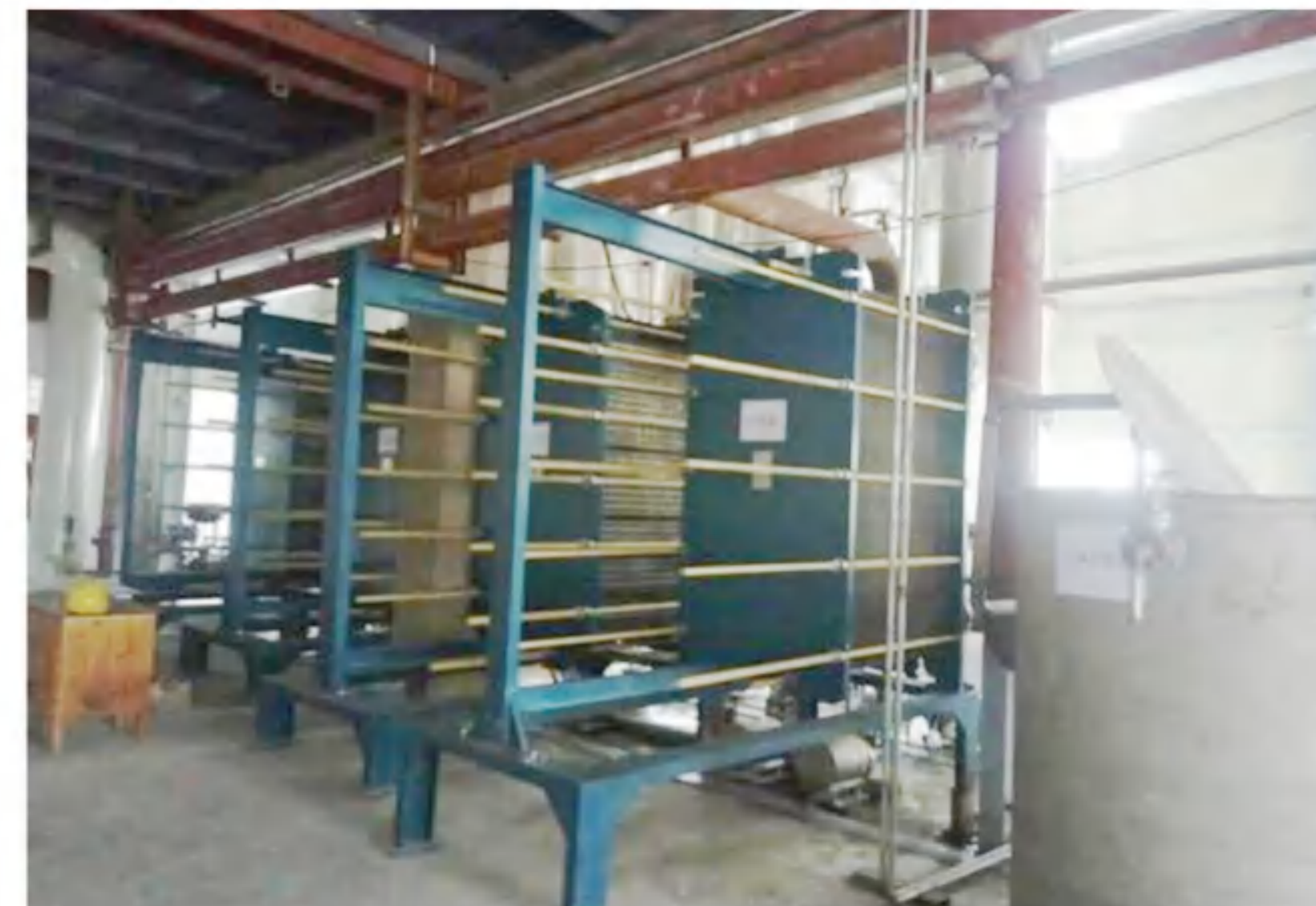
Evaporation capacity: 13t/h Evaporation process: Three effect evaporation Fluid: Refined sugar Final concentration: 75% Main material: SS316L
