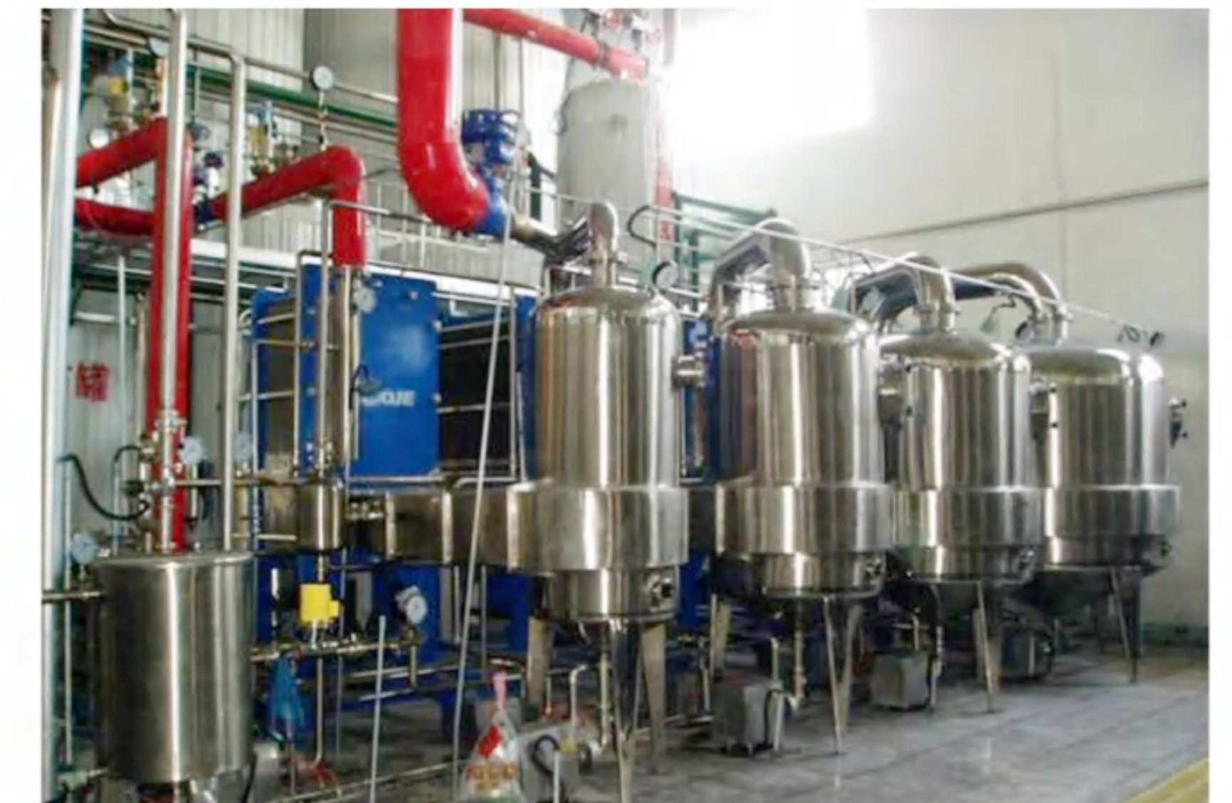
Evaporation capacity: 20t/h Evaporation process: 4 effect evaporation Fluid: Maltose Final concentration: 77% Main material: SS316L
