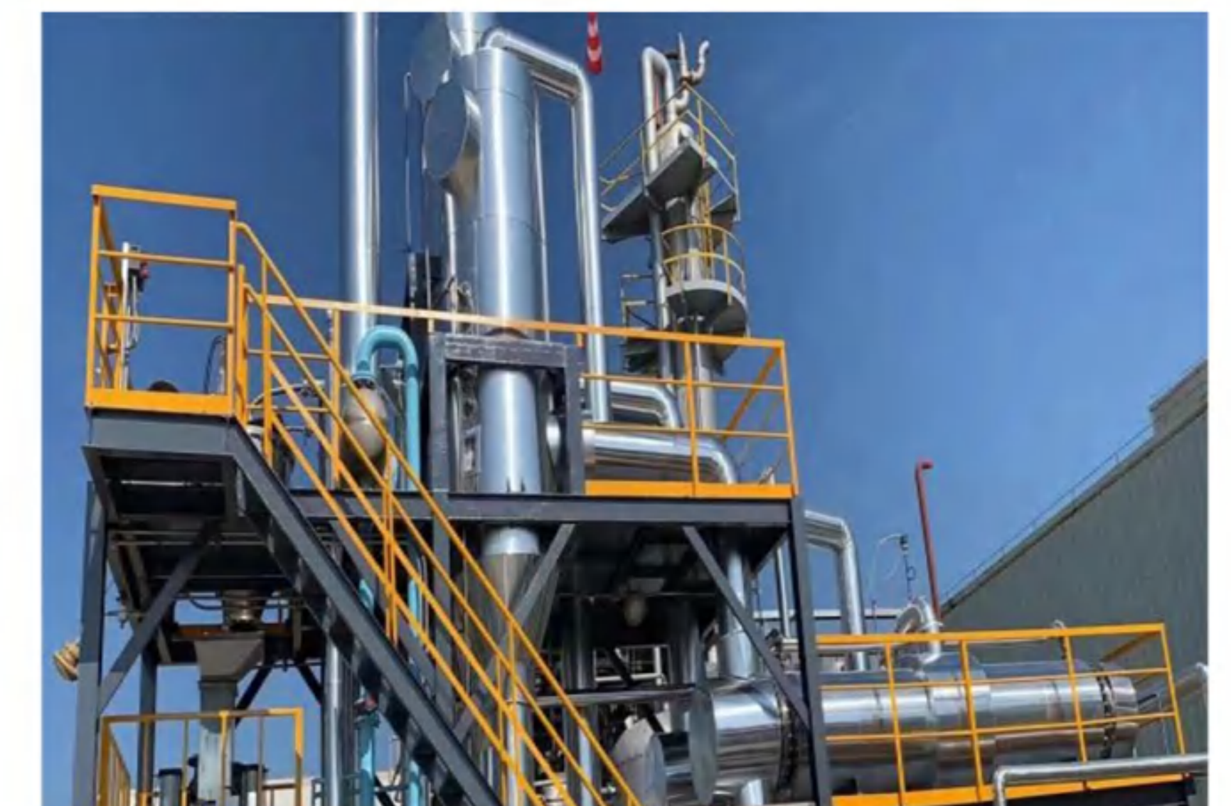
Evaporation: 1.4t/h Process: Double-effect tube force circulation+packing unit Material: Na 2 SO 4 Final concentration: Crystallization Main material: 316L
