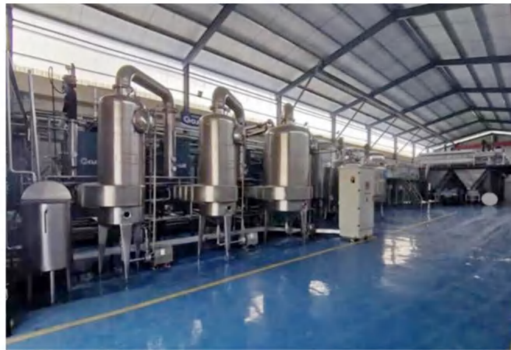
Evaporation capacity: 6t/h Evaporation process: Three effects Material: Pectin Final concentration: 10% Main material: SS316L
