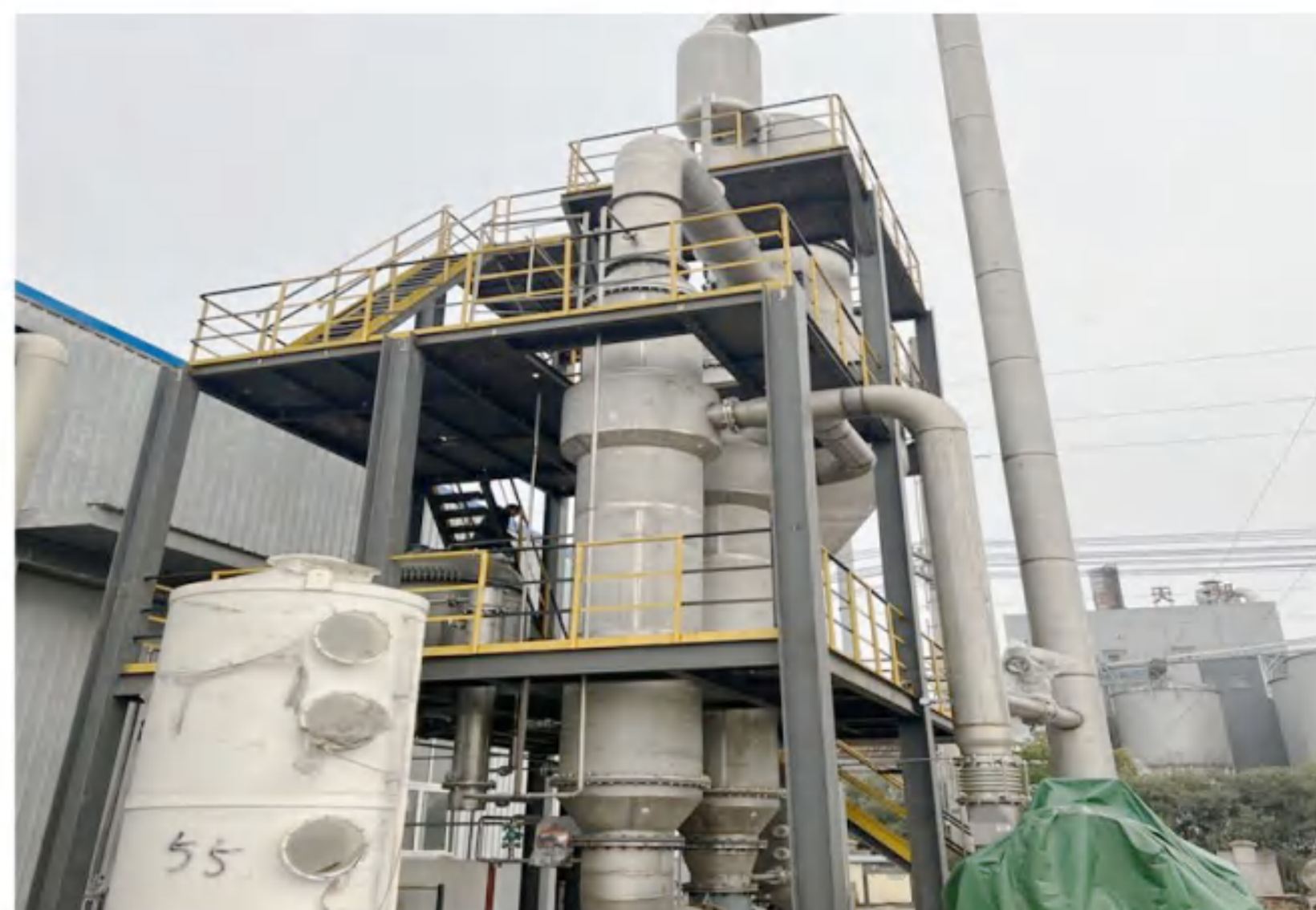
Evaporation capacity 4.13t/h Evaporation process: MVR evaporation crystallization Material: Manganese sulfate Main material: TA2
