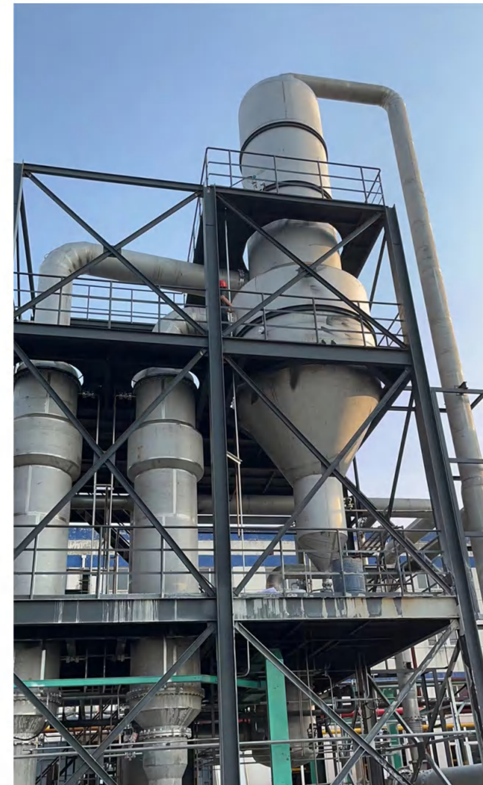
Evaporation capacity: 10t/h Evaporation process: MVR falling film + forced cycle evaporation crystallization Fluid: potassium sulfate Final concentration: 10% Main material: SS316L
