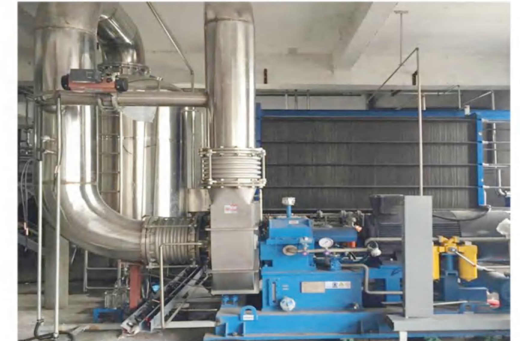
Evaporation capacity: 7t/h Evaporation process: MVR single effect Fluid: Low temperature fructose Final concentration: 75% Main material: SS316L
