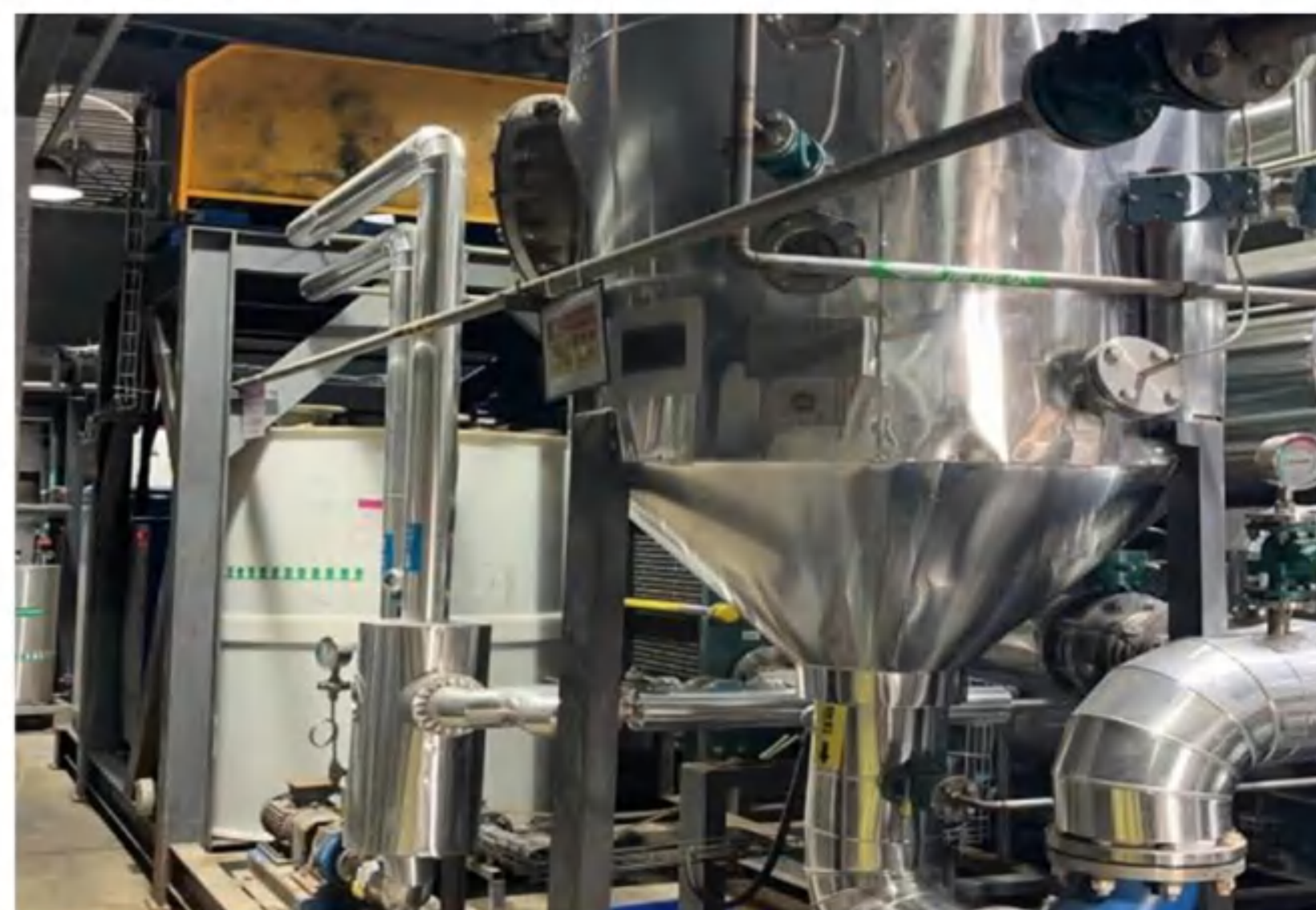
Evaporation: 1.6t/h Evaporation process: Pretreatment + MVR evaporation system Materials: High-salt wastewater Final concentration: Crystallization Main material: TA2
