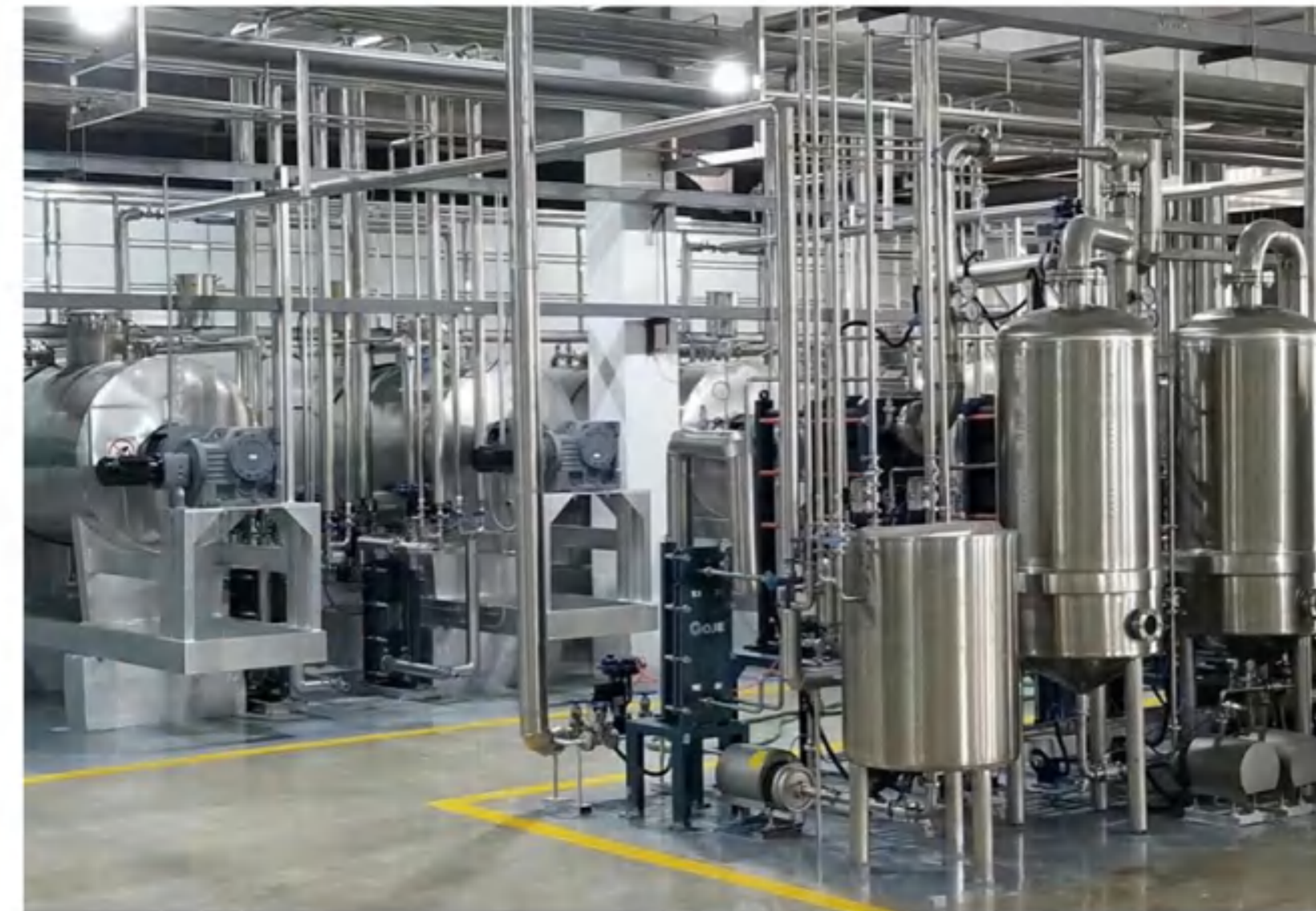
Evaporation capacity: 2t/h Evaporation process: Two effect Fluid: Glucose Final concentration: 75% Main material: SS316L
