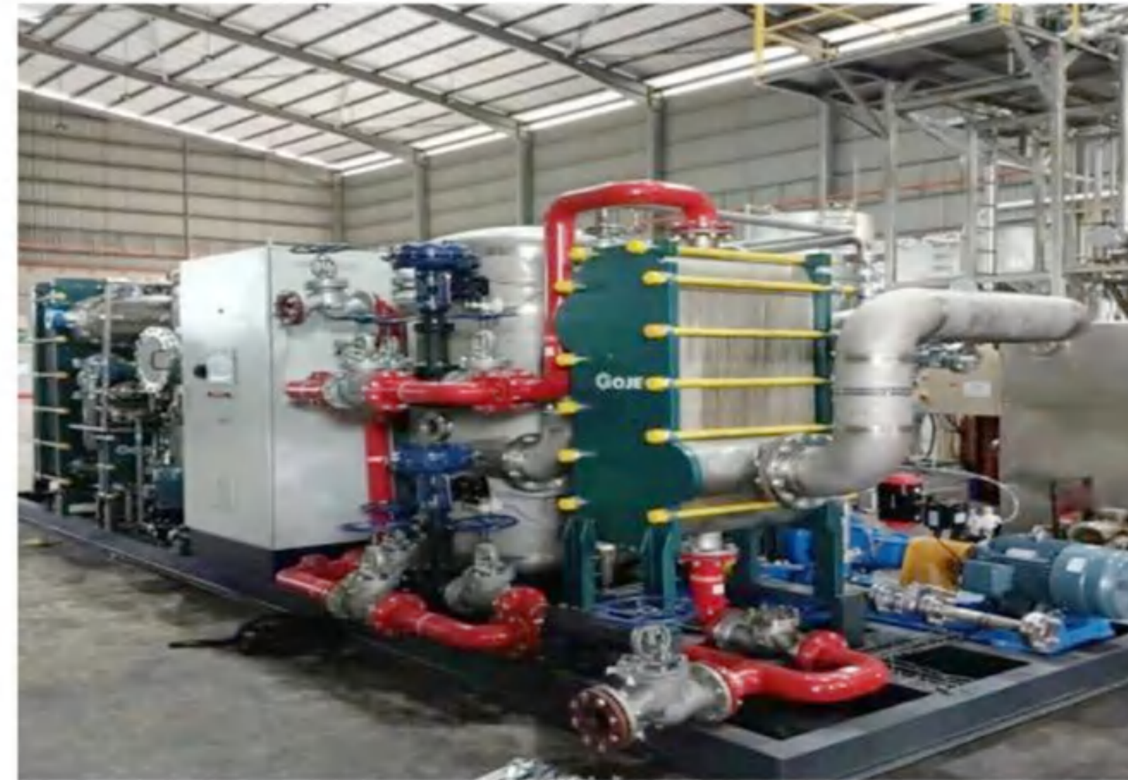
Evaporation capacity: 2.6t/h Evaporation process: Three effects Fluid: Oat milk Final concentration: 80% Main material: SS304
