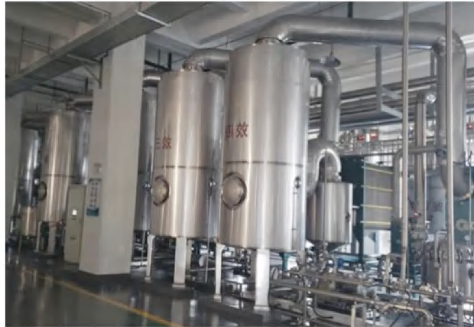
Evaporation capacity: 20t/h Evaporation process: four effects Material: Sugar solution Final concentration: 77% Main material: SS316L
