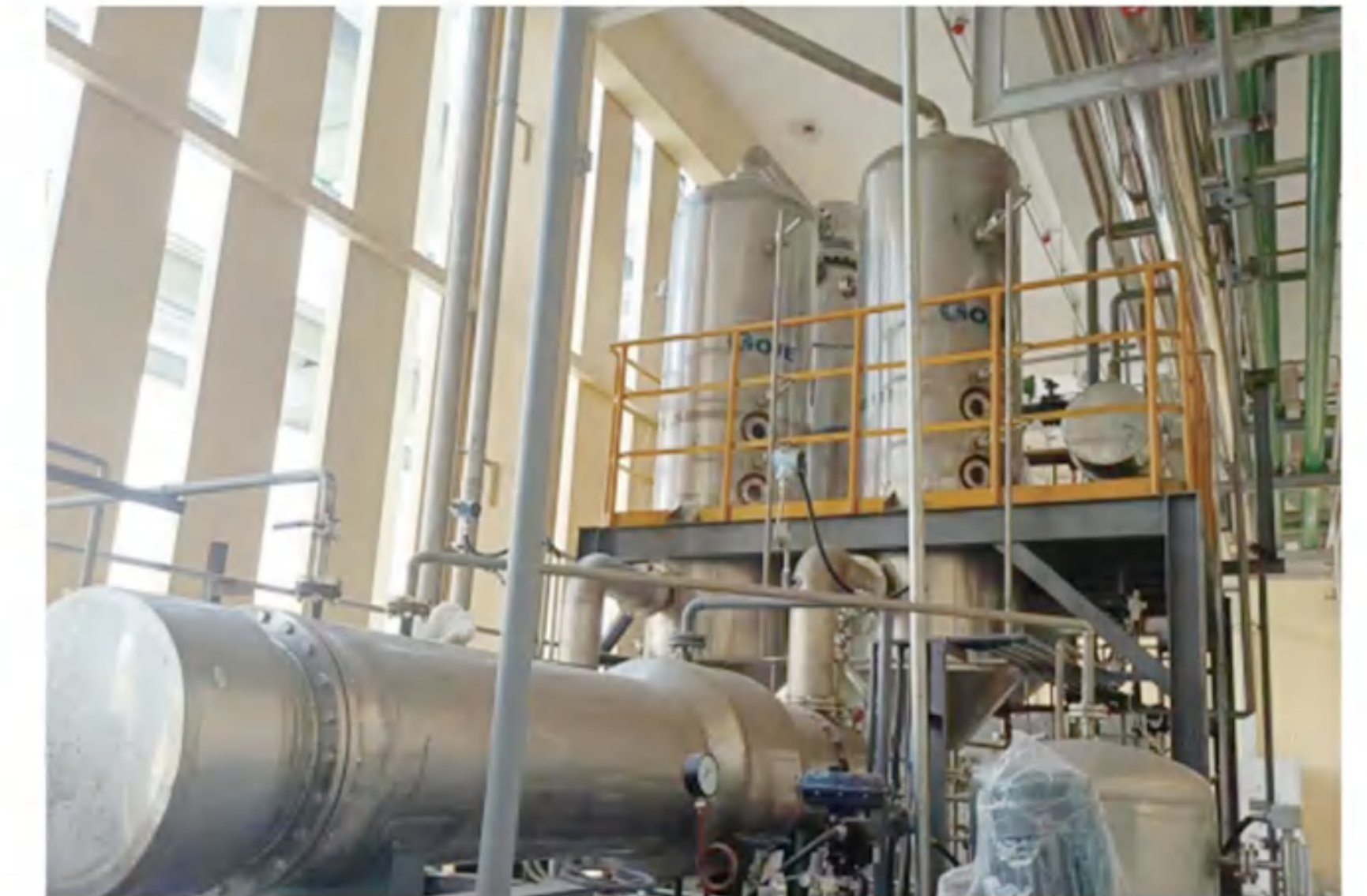
Evaporation capacity: 0.85t/h Evaporation process: Two effect evaporation crystallization system Fluid: Sodium chloride and ammonium chloride Main material: 2205
