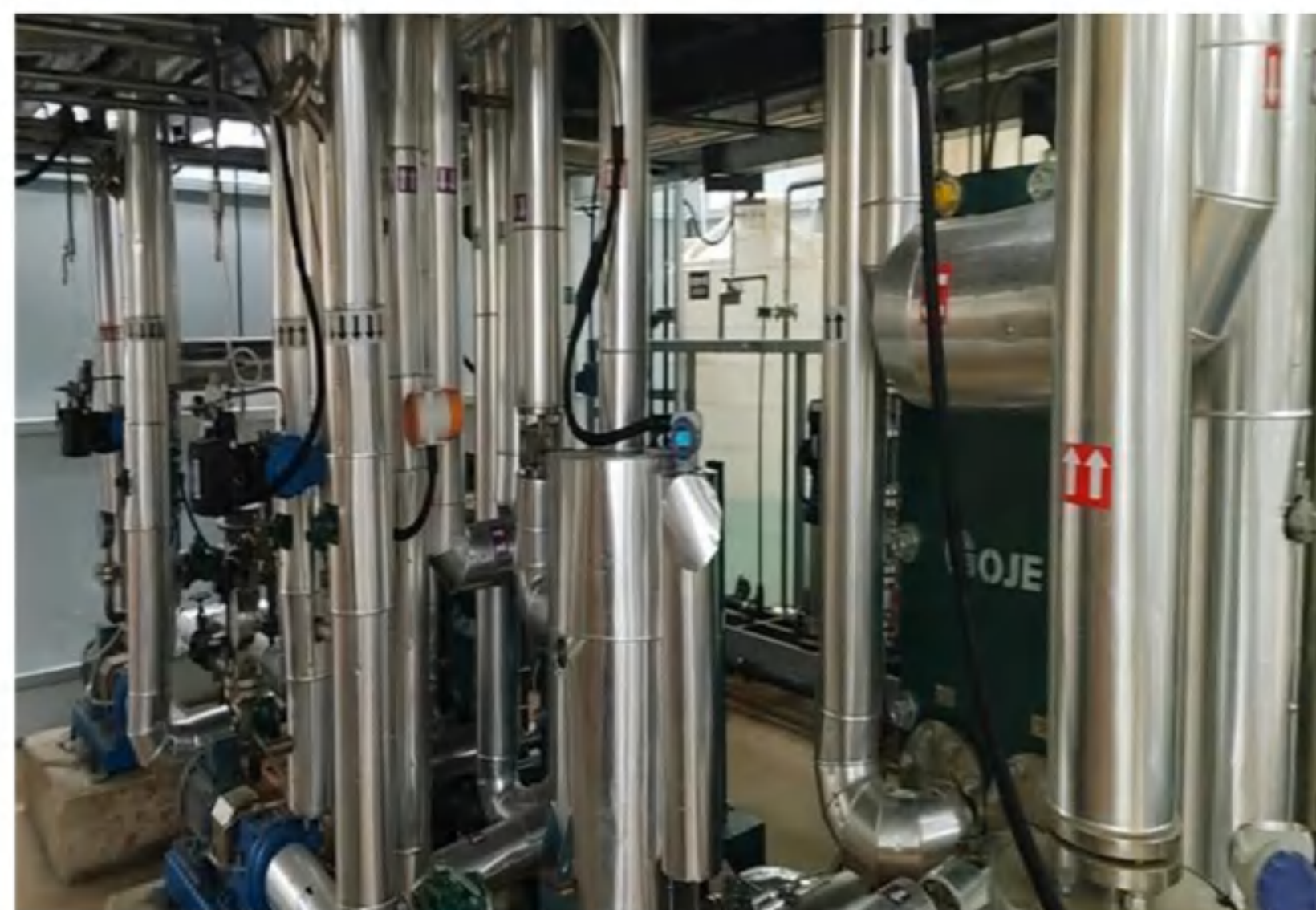
Evaporation: 2.6t/h Evaporation process: two-effect plate climbing film + tube forced circulation Material: sodium chloride (waste water) Final concentration: crystallization Main material: TA1 TA2
