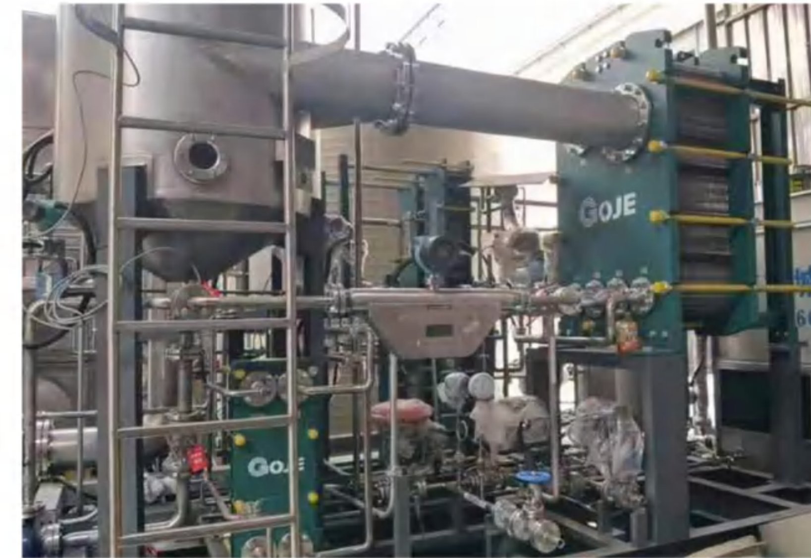
Evaporation: 1t/h Process: MVR plate rising film evaporation system Material: Pickling wastewater Final concentration: 50% Main material: 904L
