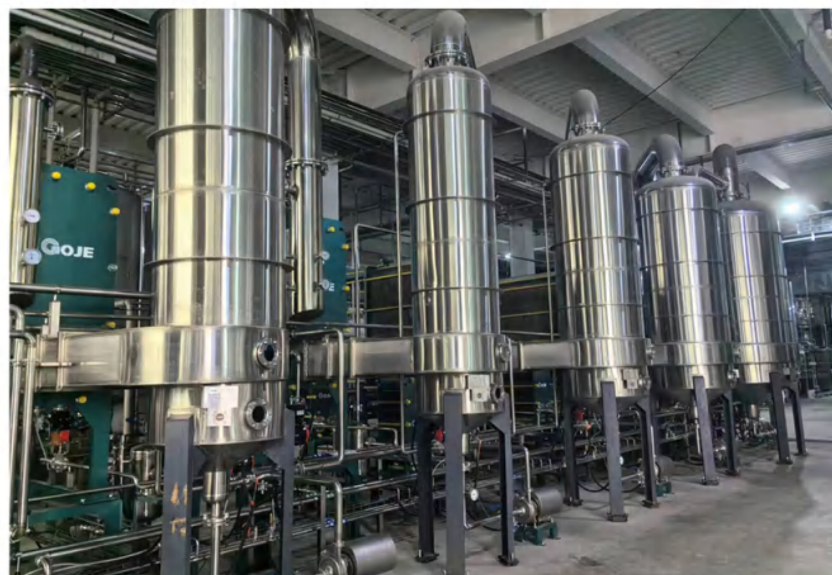
Evaporation capacity: 10t/h Evaporation process: MVR plate evaporation system Fluid: Juice Discharge concentration: 75% Main material: S30403
