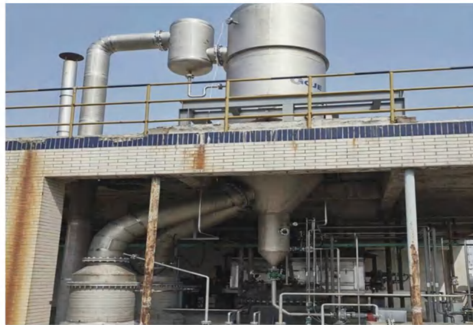
Evaporation capacity: 3t/h Evaporation process: MVR+ single effect evaporation crystallization Fluid: Sodium chloride sodium sulfate mixture Main material: TA2
