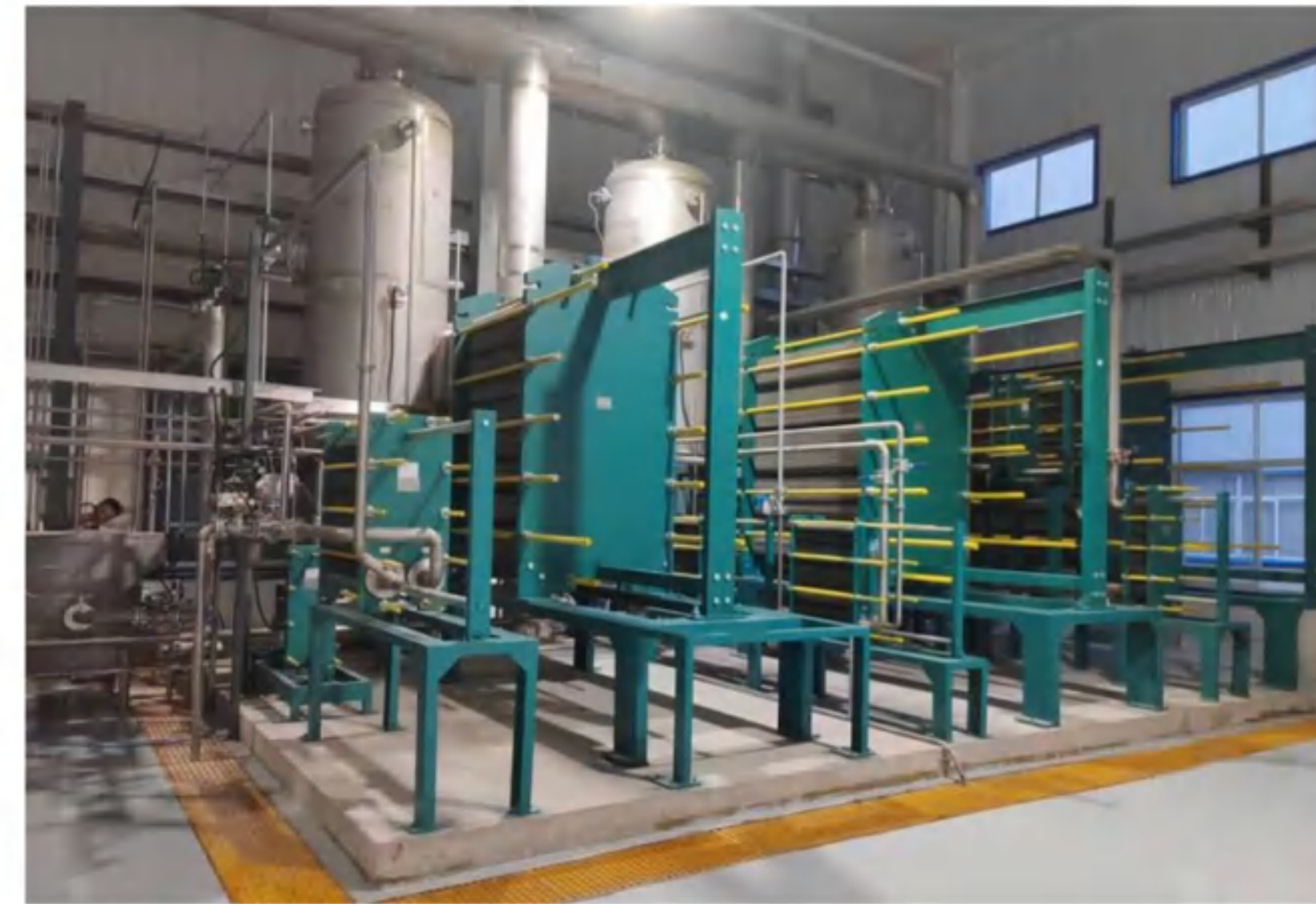
Evaporation: 18t/h Process: MVR triple-effects plate evaporation system Material: NaOH Final concentration: 21.7% Main material: 316L
