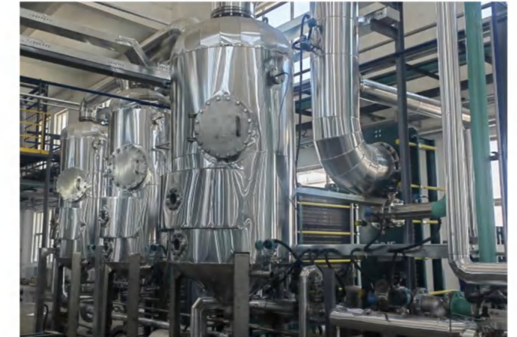
Evaporation: 3.62t/h Evaporation process: three-effect plate Material: hydrolyzate Discharge concentration: 65% Main material: 316L
