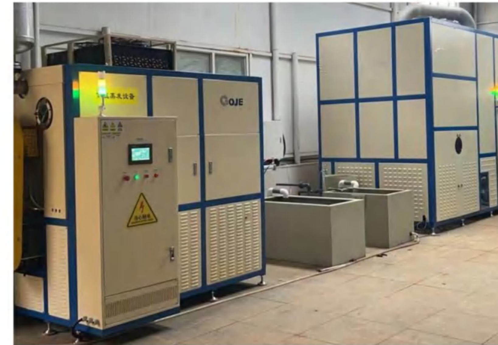
Evaporation capacity: 7t/d Evaporation process: low-temperature heat pump evaporation crystallization Fluid: electroplating wastewater (galvanized oily wastewater, chromium wastewater, nickel wastewater, copper wastewater) Final concentration: Crystallization Main material: TA2
