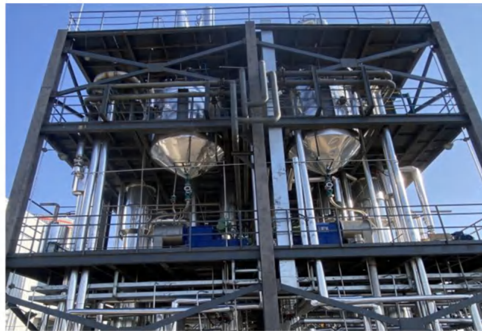
Evaporation: 3.5 t/h 2.5 t/h Evaporation process: 2 sets of triple-effects tube forced circulation evaporation system Material: NaCl, NaBr Final concentration: Crystallization Main material: TA2
