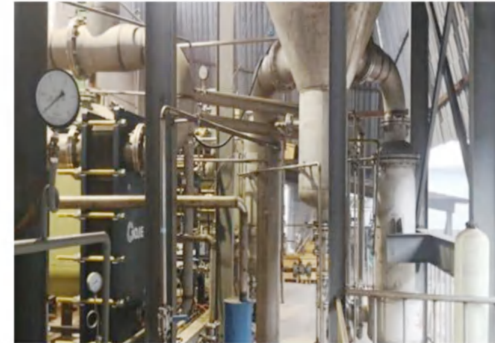
Evaporation capacity: 2t/h Evaporation process: Two effect evaporation crystallization Fluid: Pickling wastewater Final concentration: crystallize Main material: SS316L
