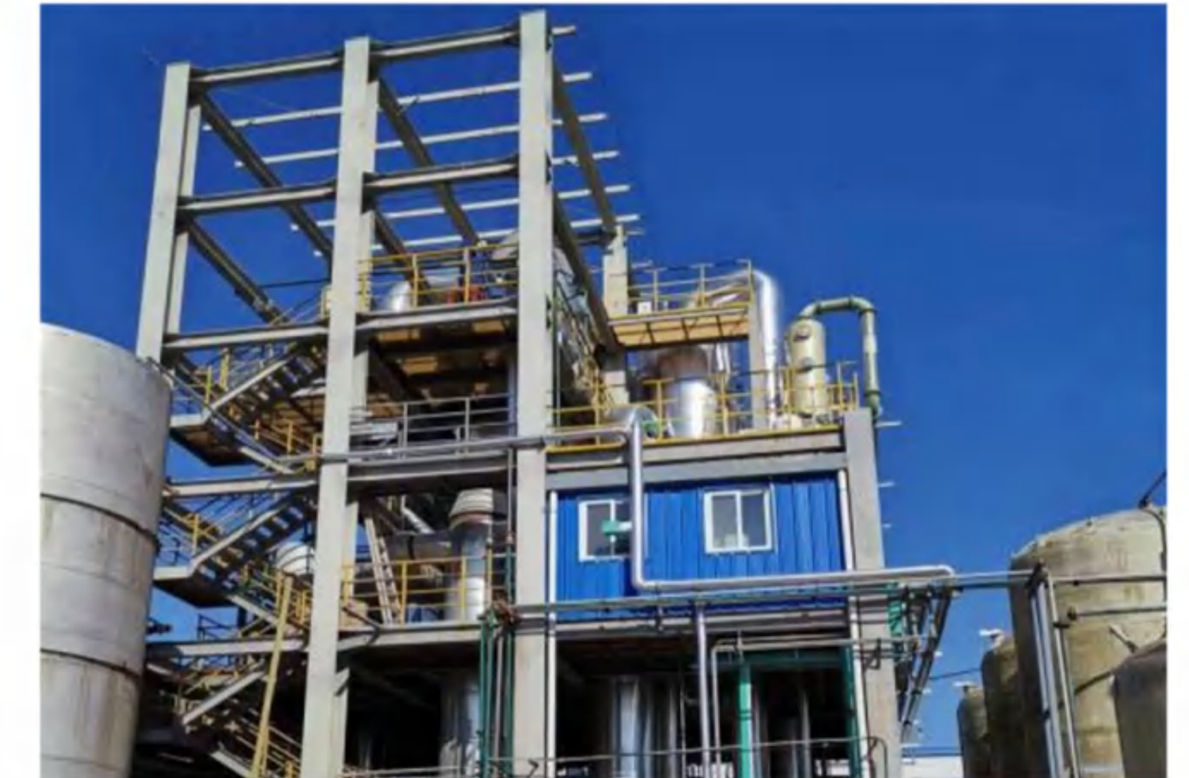
Evaporation capacity: 7.5t/h Evaporation process: MVR single effect evaporation crystallization Material: Sodium chloride Main material: TA2
