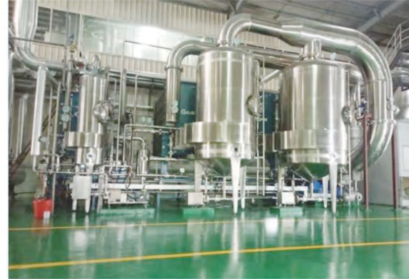
Evaporation capacity: 10t/h Evaporation process: MVR single effect+multi effect Fluid: Isomaltoligosaccharide Final concentration: 75% Main material: SS304
