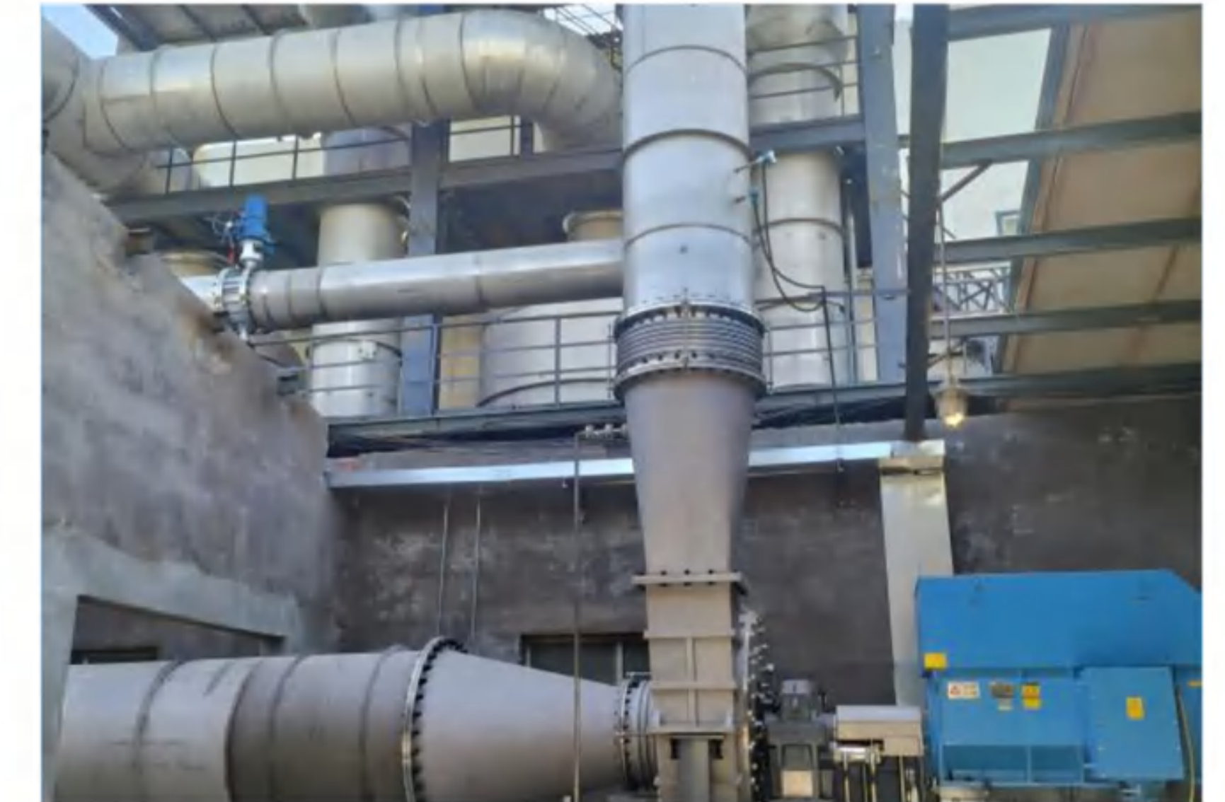
Evaporation: 10t/h Evaporation process: MVR falling film evaporation system Material: hyaluronic acid Final concentration: Crystallization Main material: 316L
