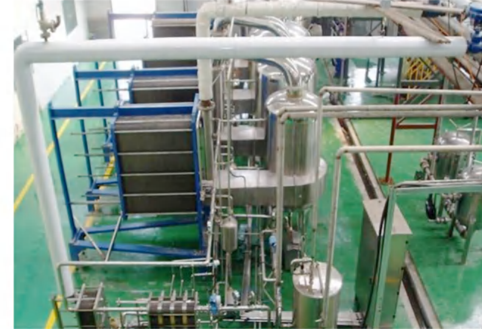
Evaporation capacity: 20t/h Evaporation process: Four effect Fluid: Oligofructose Final concentration: 75% Main material: SS316L
