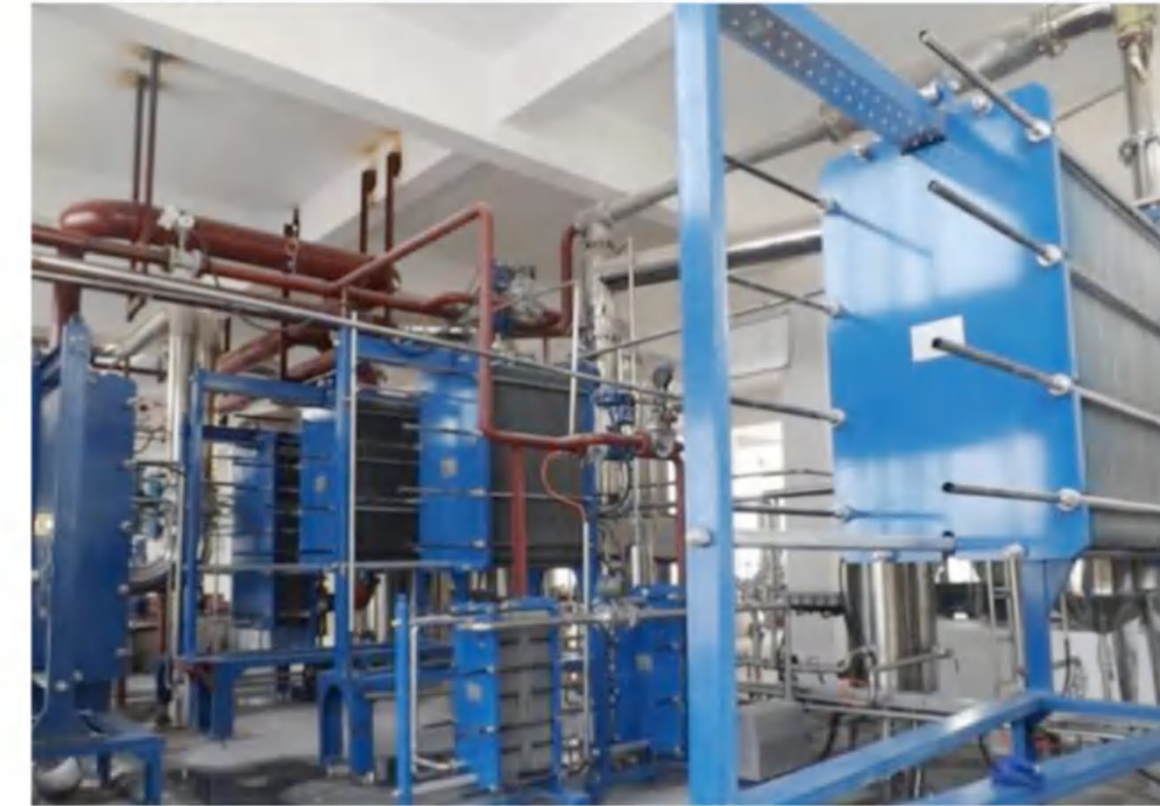
Evaporation capacity: 10t/h Evaporation process: TVR triple effect + column tube Fluid: Gluconolactone Final concentration: 85% Main material: SS316L
