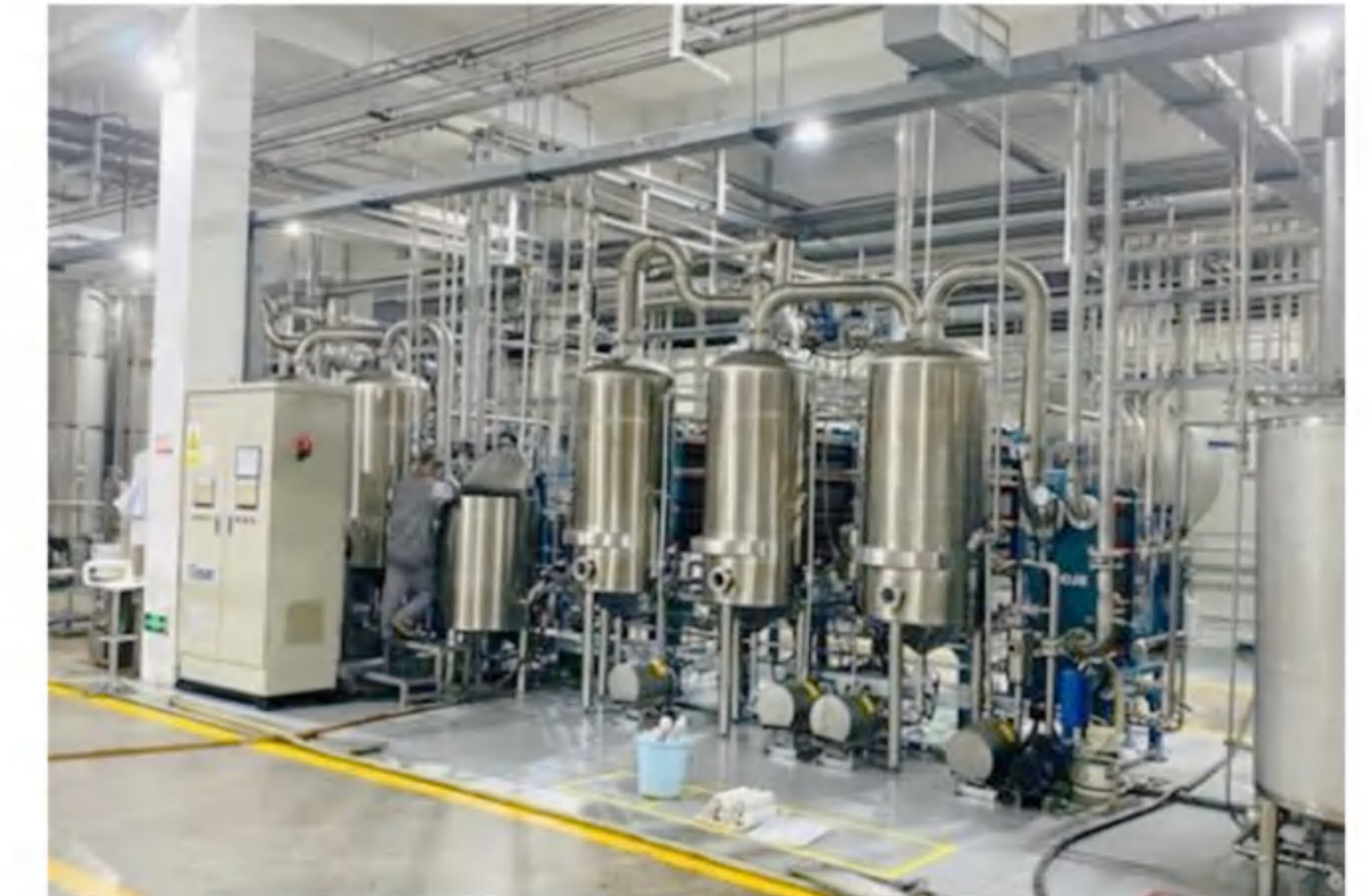
Evaporation capacity: 2t/h Evaporation process: Multi - set multi - effect Fluid: Glucose, polysaccharide Final concentration: 75% Main material: SS316L
