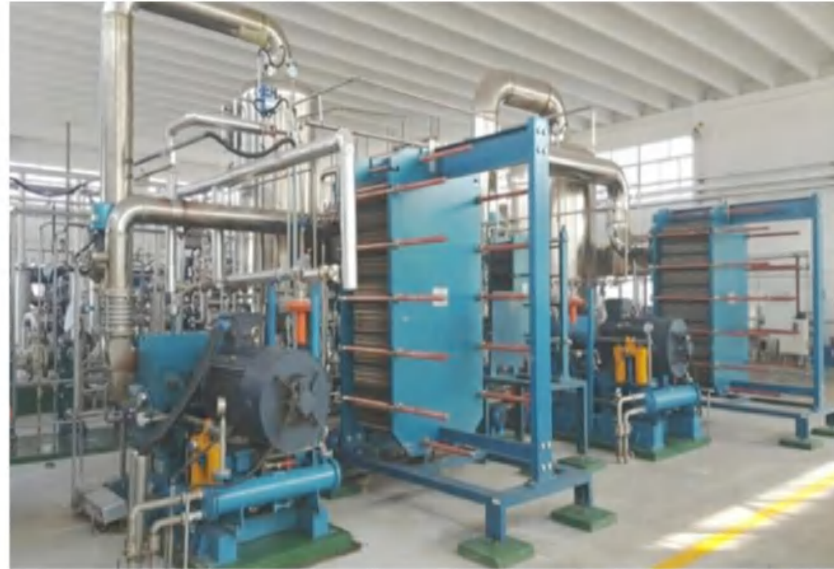
Evaporation capacity: 3t/h Evaporation process: MVR single effect+multi effect Fluid: Lactic acid Final concentration: 85% Main material: Ti
