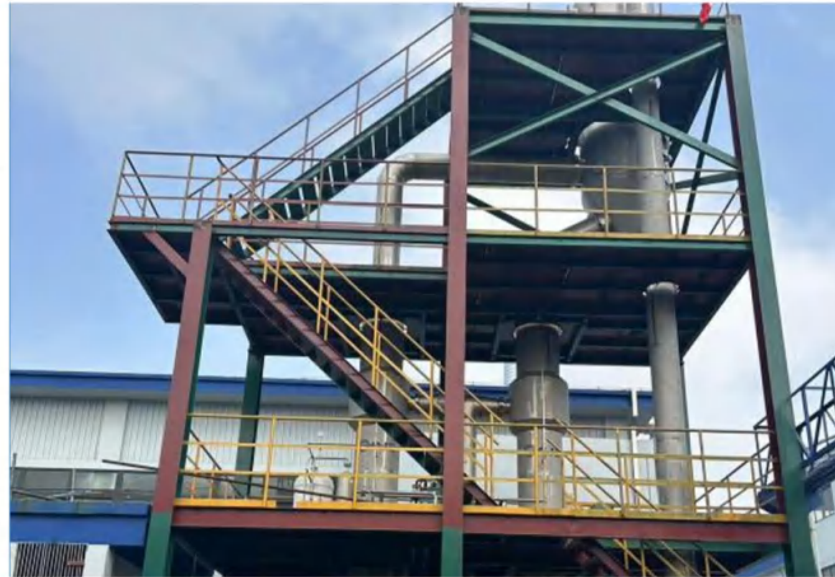
Evaporation: 2.6t/h Evaporation process: MVR tube evaporation system Material: zinc sulfate heptahydrate Final concentration: frozen crystallization Main material: 2507
