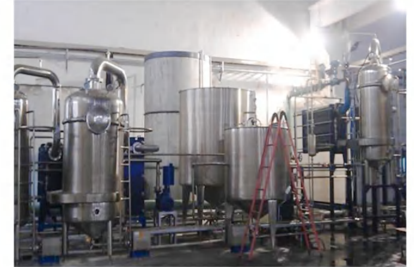
Evaporation capacity: 4t/h Evaporation process: 3+1 effect flash evaporation Fluid: Polyethylene glycol Final concentration: 99.5% Main material: SS316L
