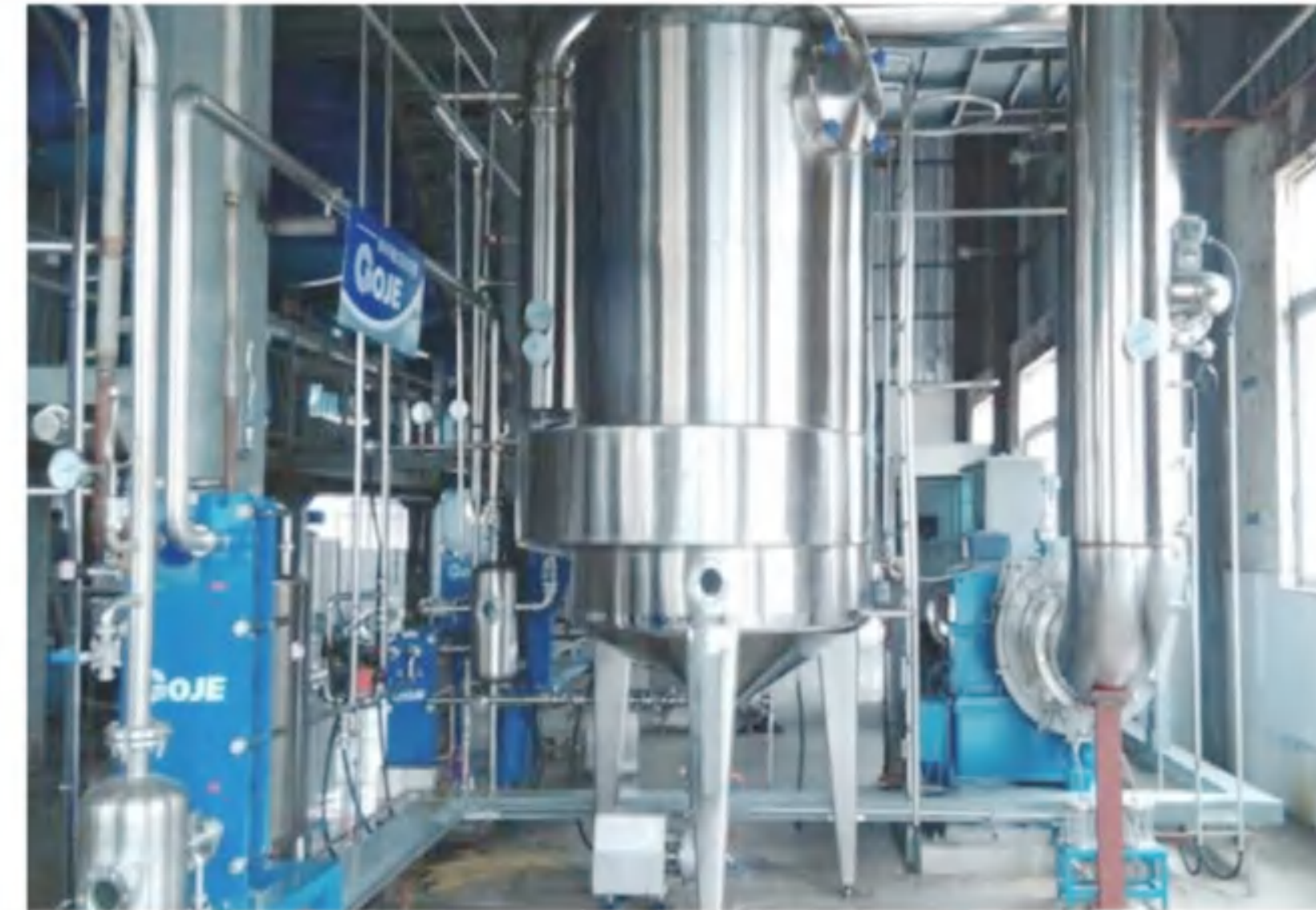
Evaporation capacity: 5t/h Evaporation process: MVR single effect Fluid: Sodium gluconate Final concentration: 70% Main material: SS316L
