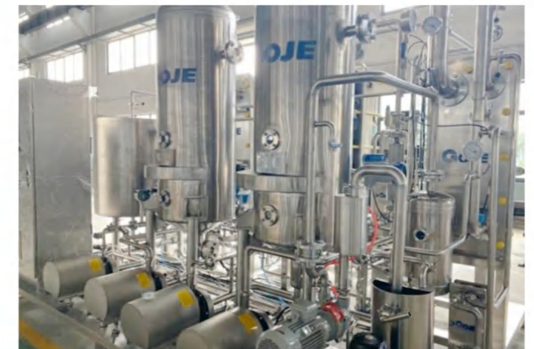
Evaporation capacity: 0.5t/h Evaporation process: two effects Fluid: Arabinose Final concentration: 70% Main material: SS316L
