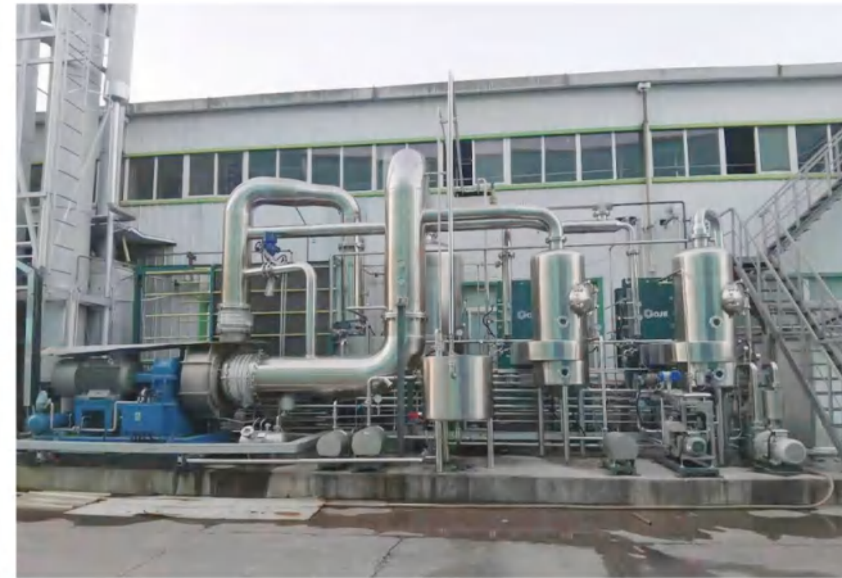
Evaporation capacity: 5t/h Evaporation process: MVR+TVR combined evaporation Material: Maltose Final concentration: 78% Main material: SS304
