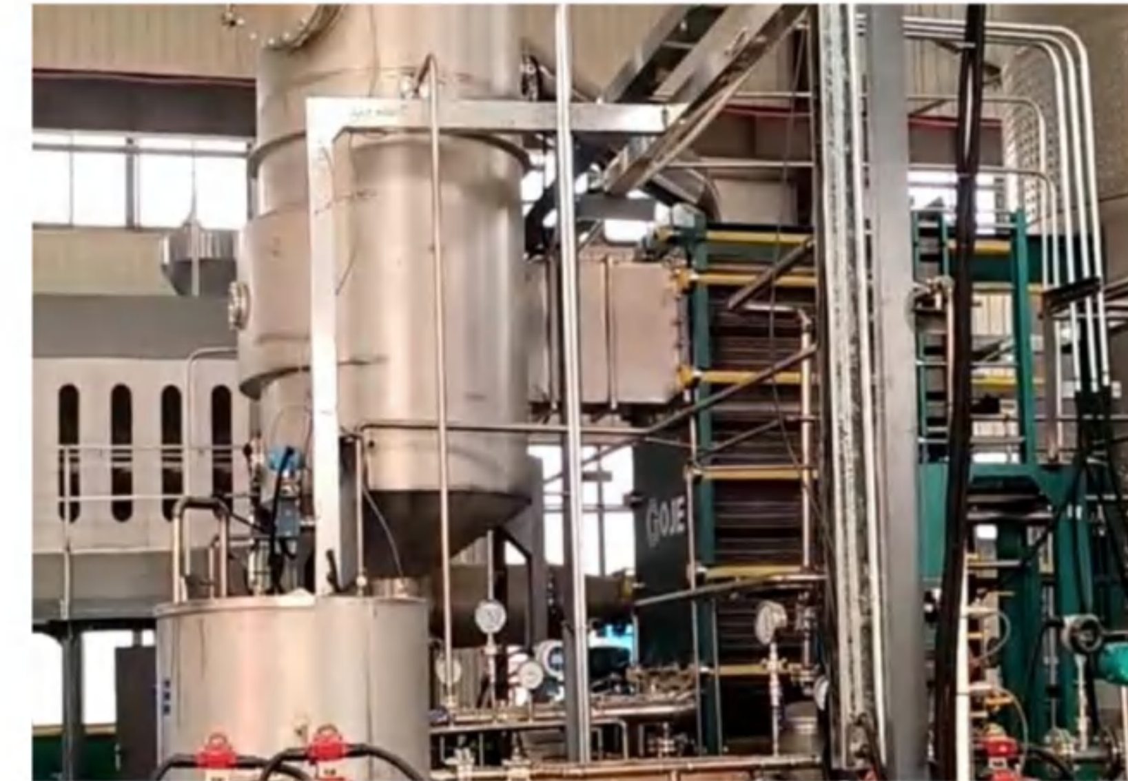
Evaporation: 2t/h Evaporation process: MVR plate evaporation concentration Material: fermented liquid of corn steep liquor Discharge concentration: 75% Main material: S31603
