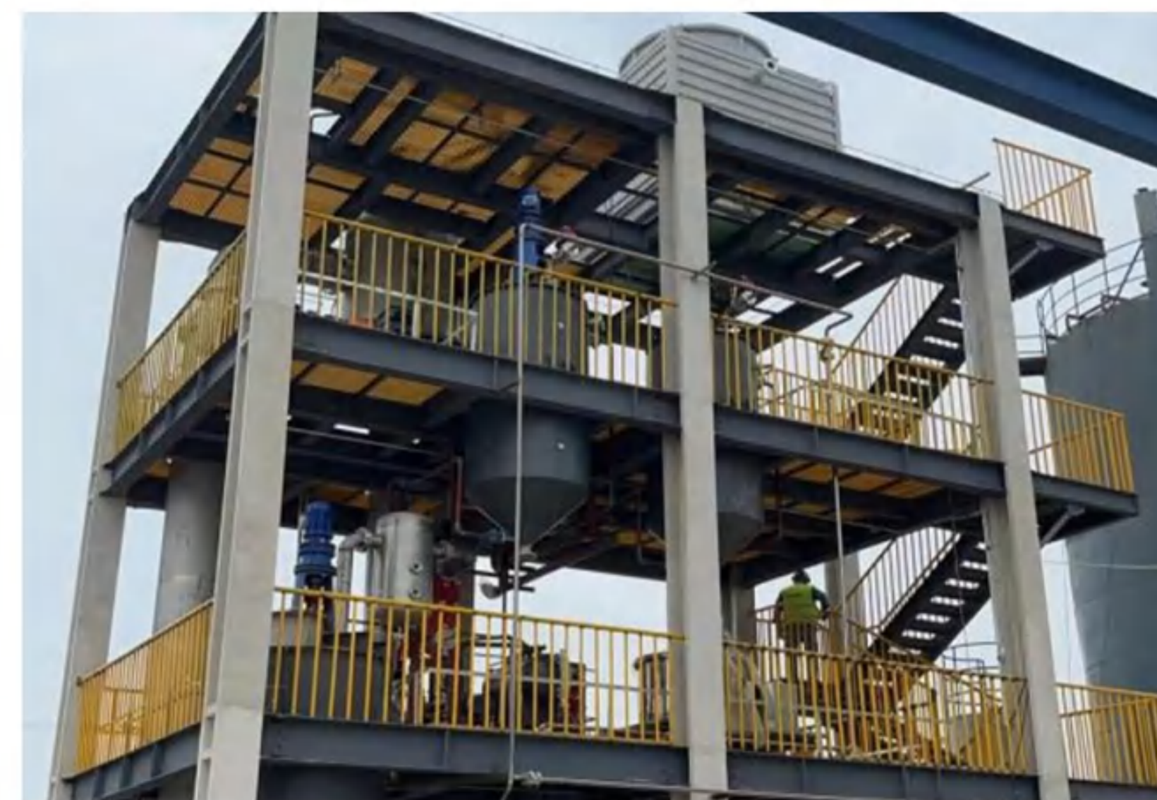
Evaporation: 1.88 t/h Evaporation process: MVR+single still evaporation system Material: NaNO 3 Final concentration: Crystallization Main material: 316L
