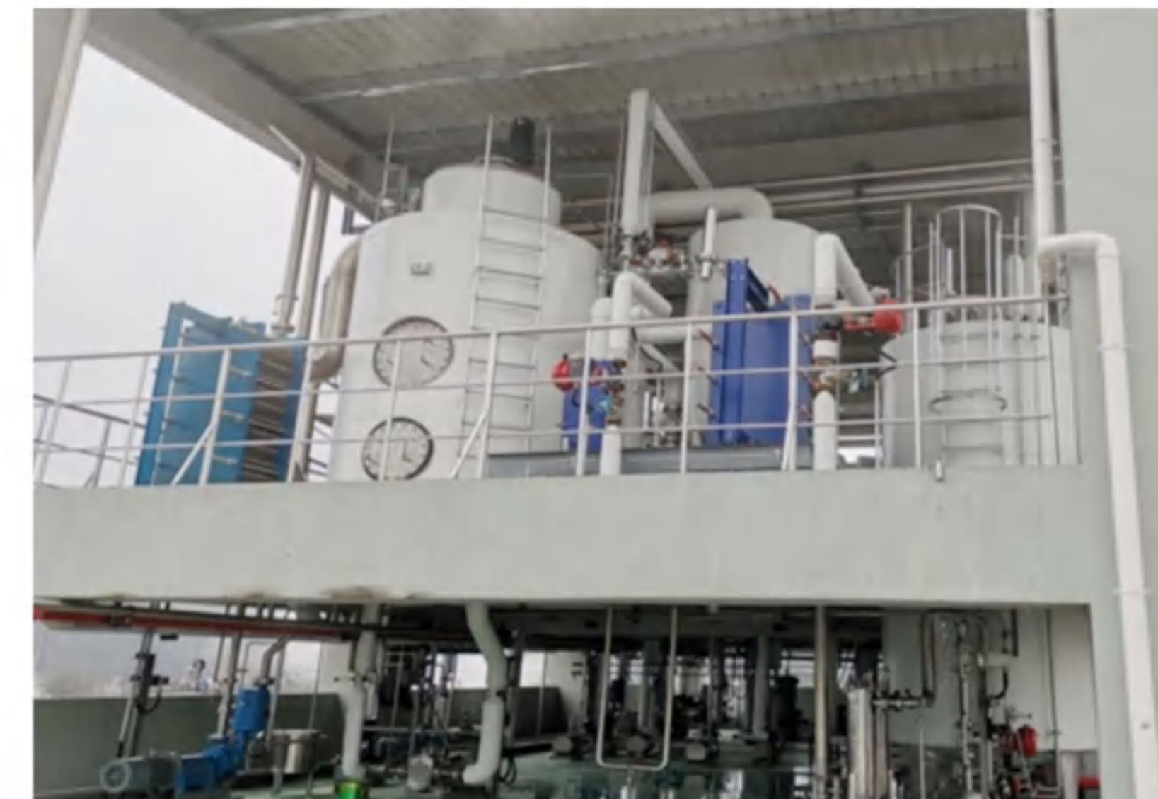
Evaporation capacity: 2t/h Evaporation process: 3 effect evaporation Fluid: Xylitol Final concentration: 82% Main material: SS316L
