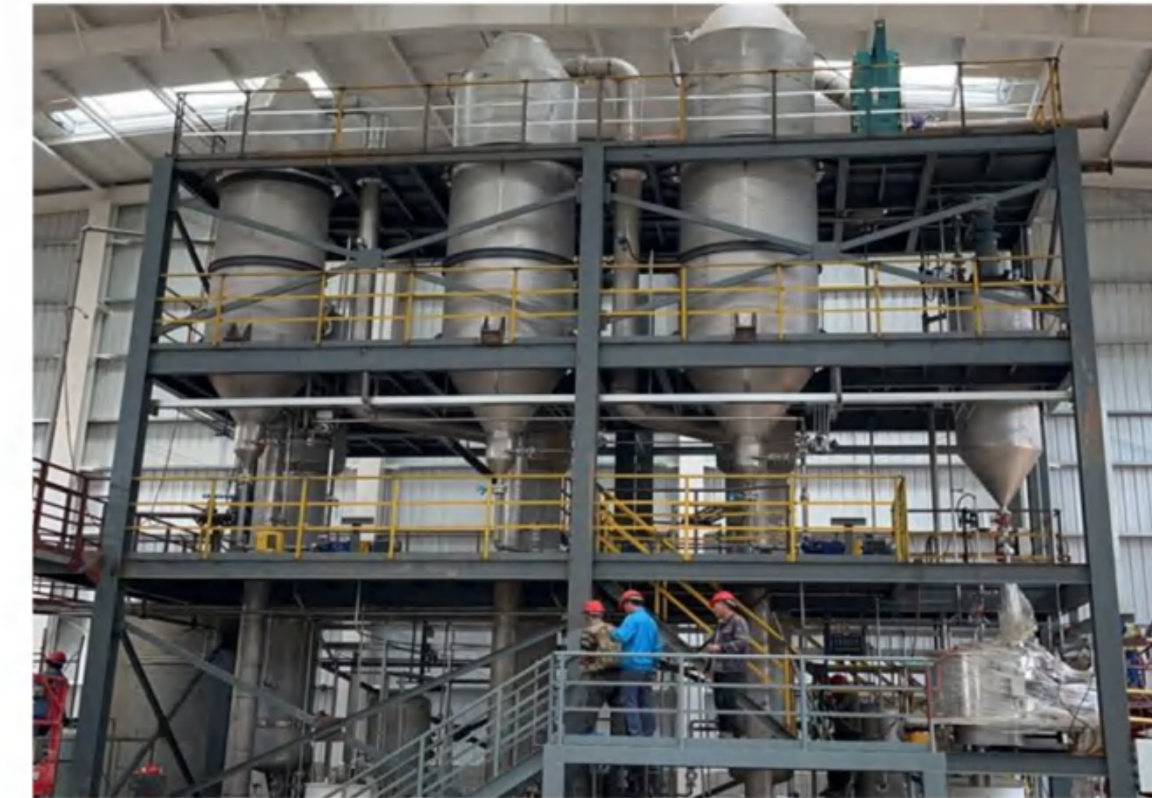
Evaporation: 5t/h Evaporation process: Triple-effect evaporation system Material: NaF Final concentration: Crystallization Main material: 316L
