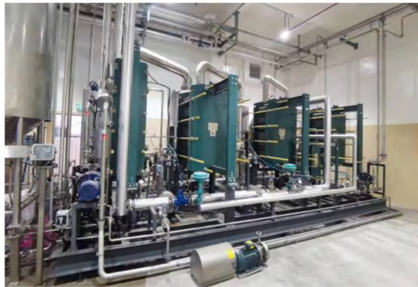
Evaporation: 3t/h Evaporation process: two-effect plate Material: waste fuel oil (waste water) Final concentration: 99% Main material: 316
