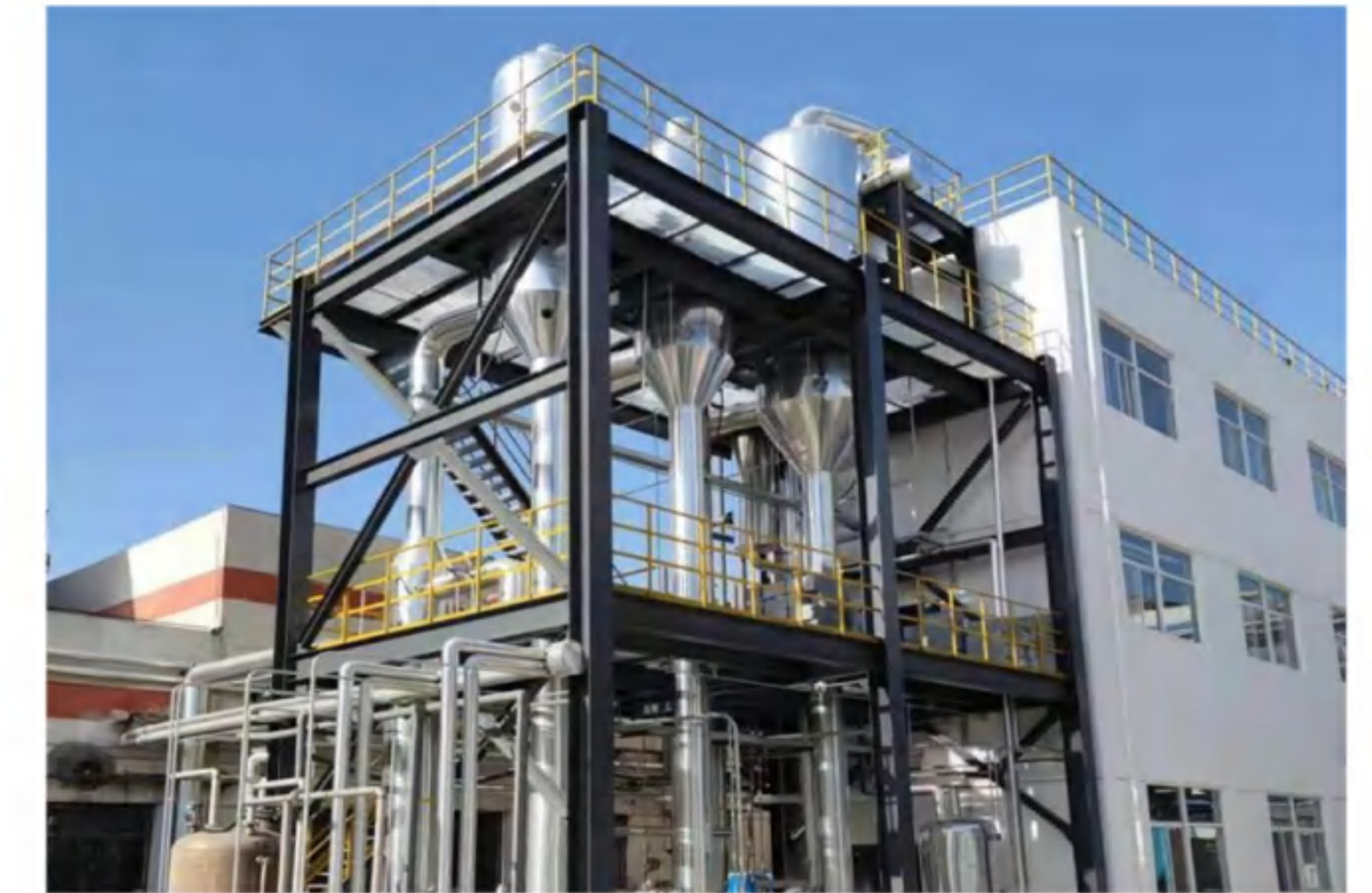
Evaporation: 3t/h Evaporation process: Triple-effect evaporation system Materials: High-salt wastewater Final concentration: crystallized salt Main material: titanium
