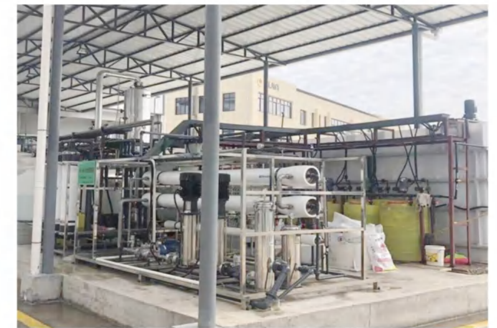
Evaporation capacity: 0.6t/h Evaporation process: Pre treatment+MVR evaporation crystallization Fluid: Wastewater Final concentration: Salt crystallization Main material: Ti
