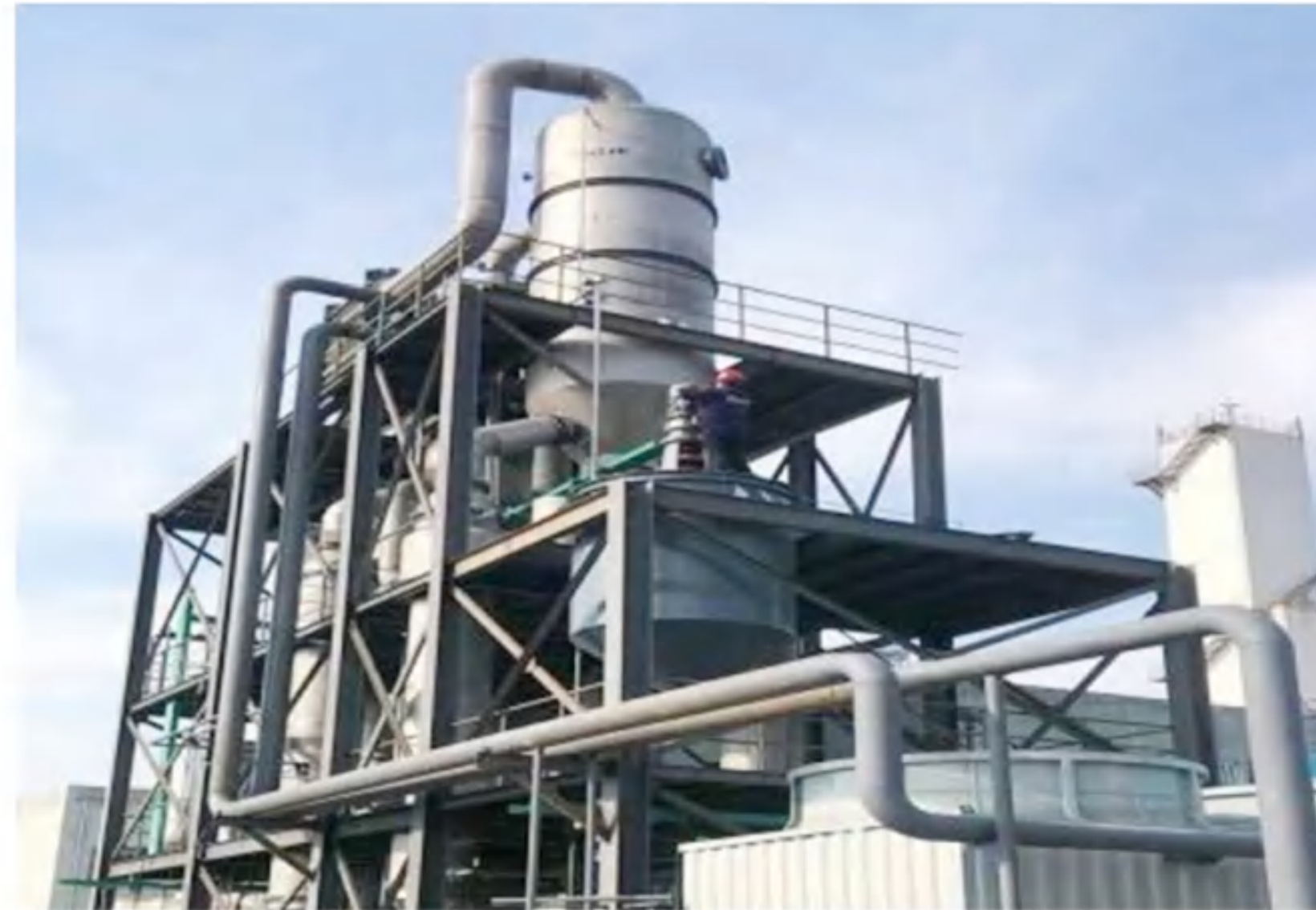
Evaporation: 10t/h Evaporation process: four-effect forced circulation Materials: sodium chloride + sodium sulfate (wastewater) Main material: TA2
