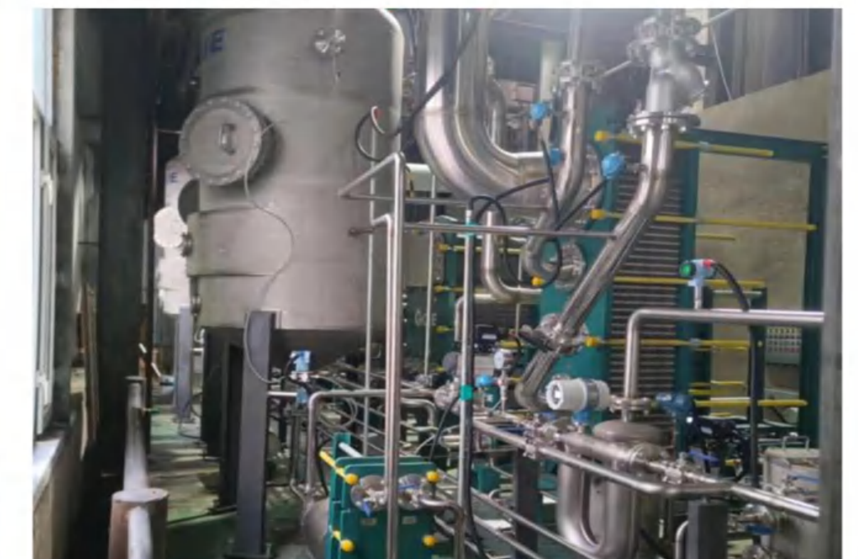
Evaporation: 4t/h Evaporation process: TVR + three-effect plate Material: Mother Liquid Sugar Final concentration: 75% Main material: 316
